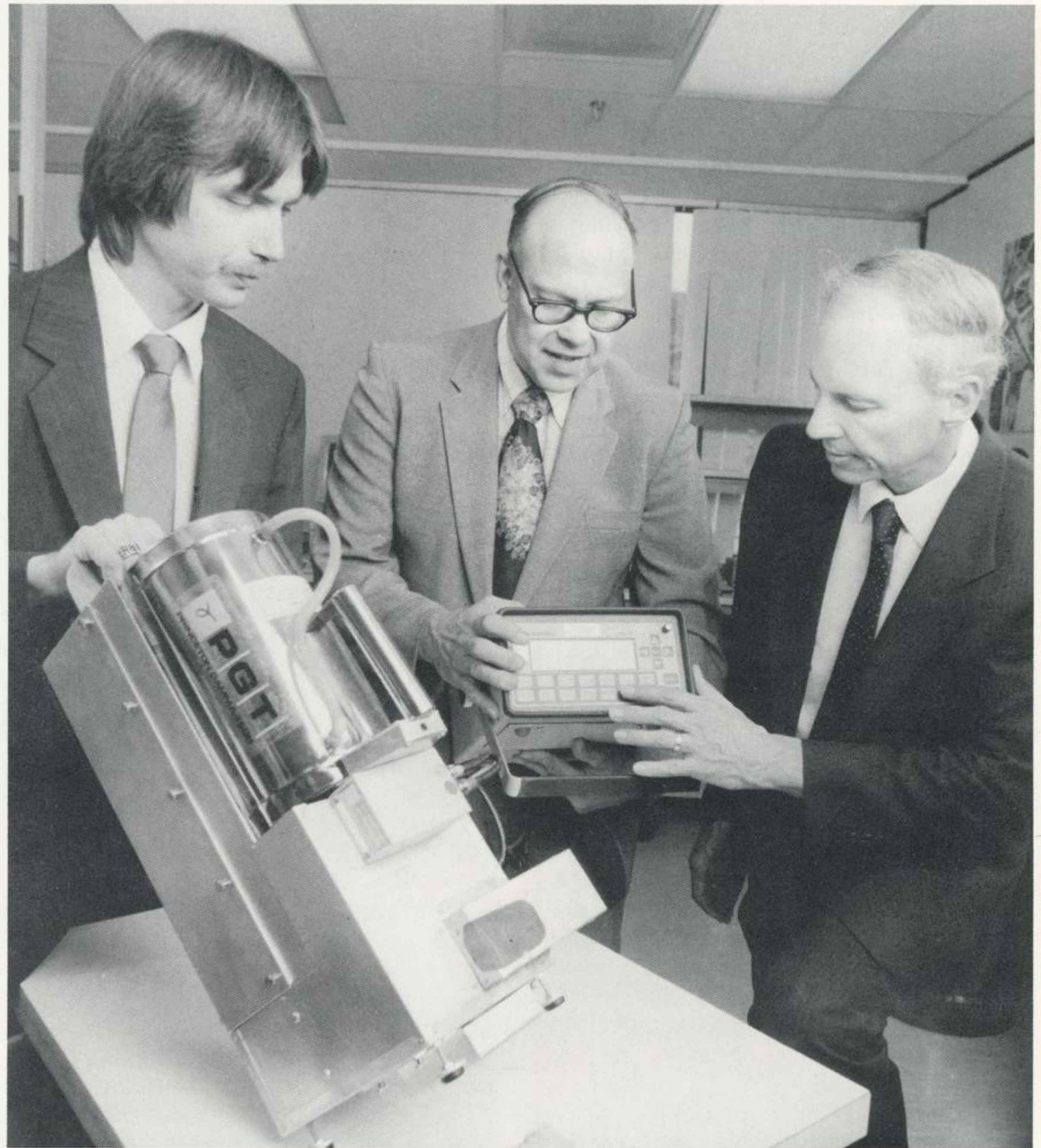
Mike Thornton, left, Warren Kelliher, center, and Benton Clark demonstrate how the hazardous waste analyzer system works. The system is designed as an on-site analysis tool for detecting the elemental composition of soils, rocks, and water.
