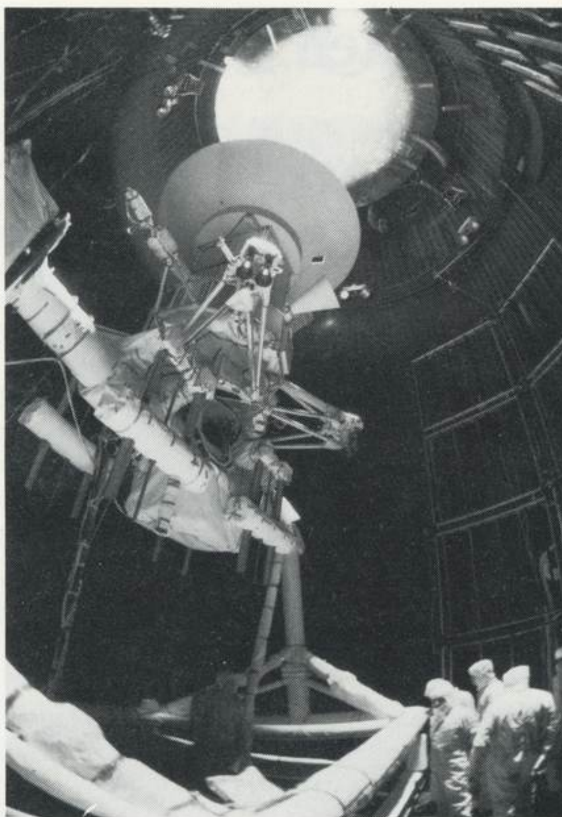
In July, the Magellan spacecraft underwent thermal vacuum testing at the Space Simulation Laboratory.
