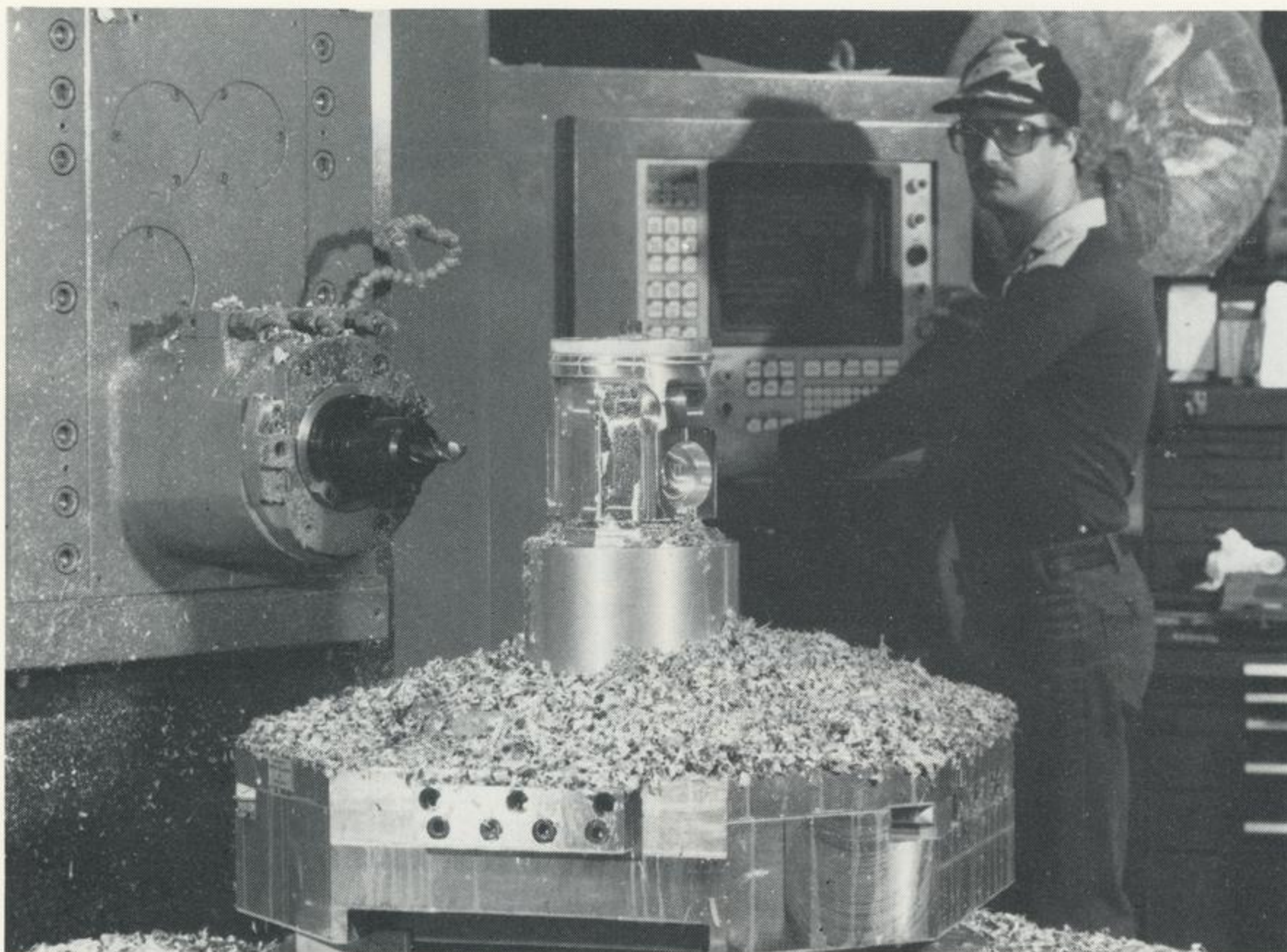
Gary W. Girardi, numerical control machinist, directs the new machining center from the control panel. The new machine is part of the continuing Manufacturing modernization.
