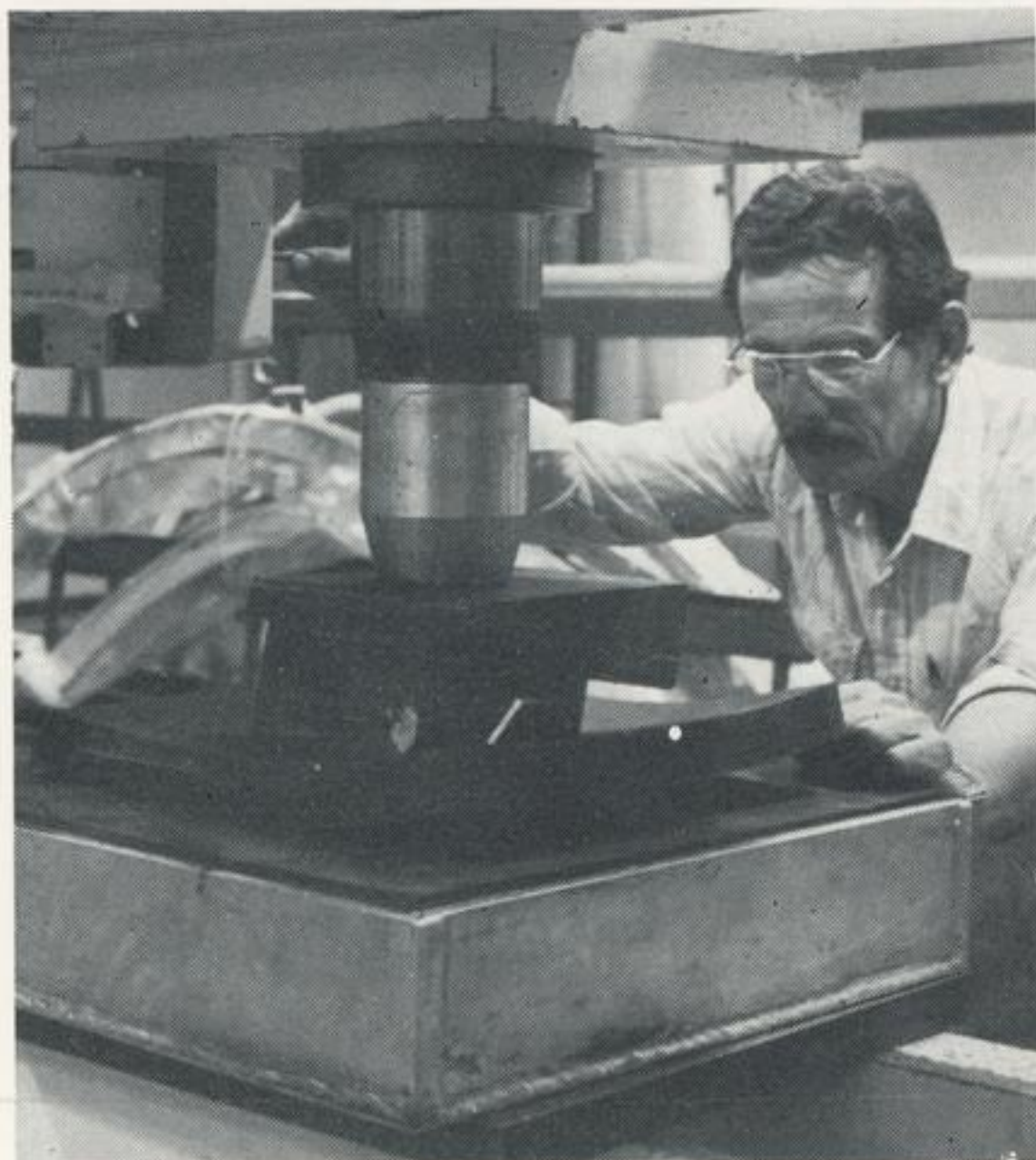
John Haney forms a Titan IV detail in a rubber box die.
