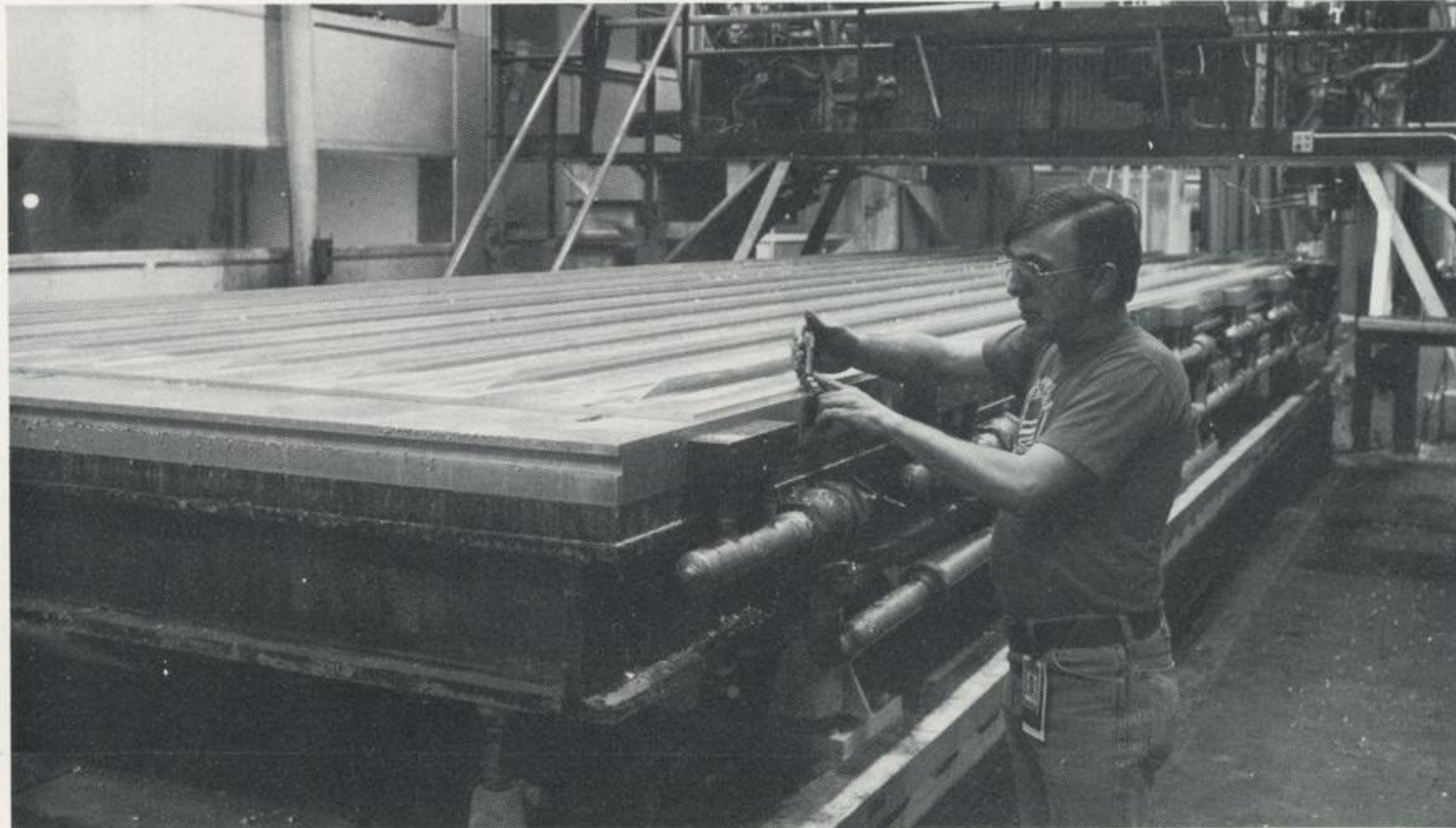
J. L. Bryant operates the skillmill during a final check of the Titan skin.
