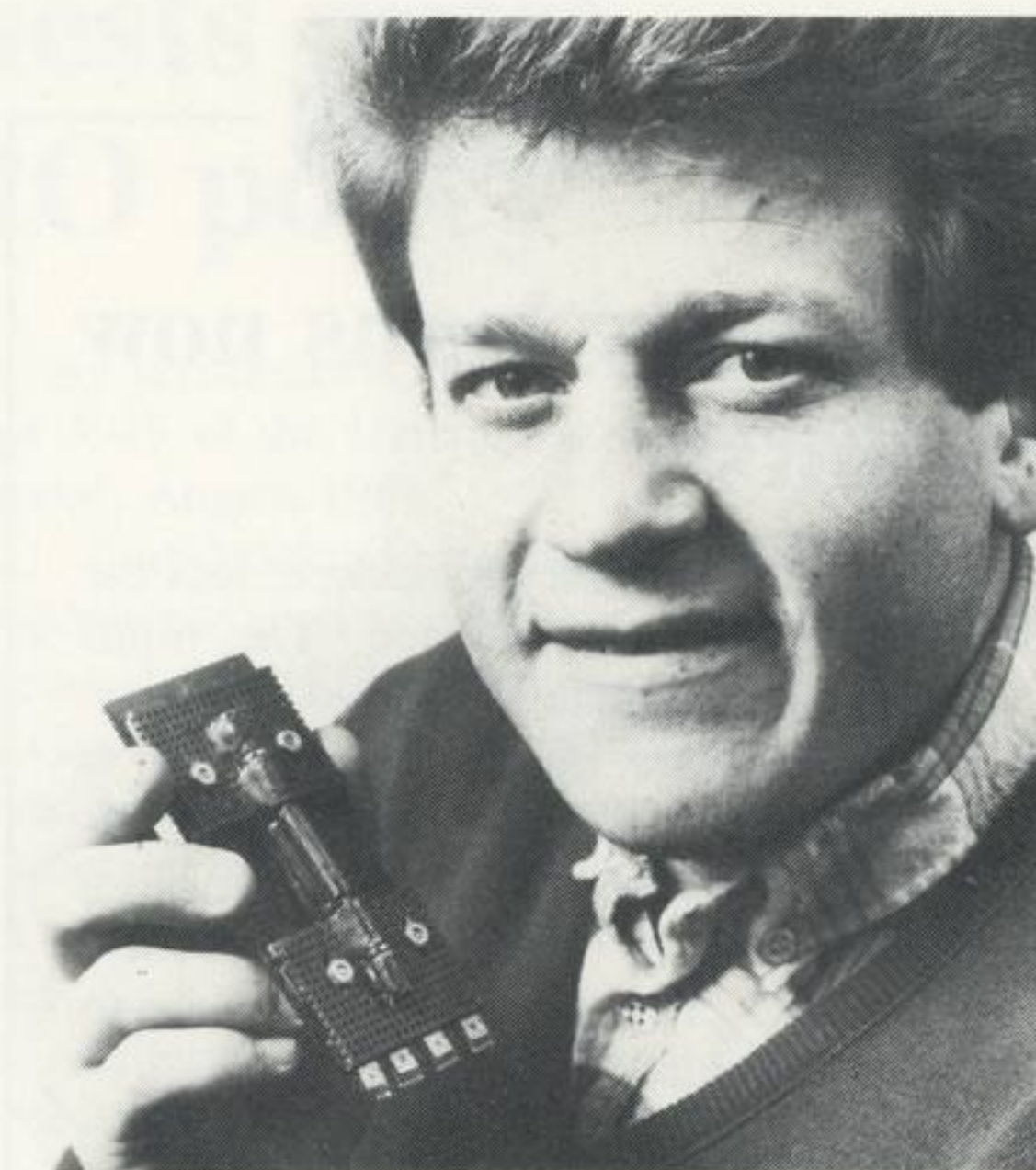
Greg Prosser shows his lead tinning tool, which adds speed and integrity to the solder-dipping process on integrated circuit flatpacks. It reduces cost and provides a more reliable product. The tool was developed under a NASA contract, the Pyrotechnic Initiator Controller (PIC) program.
