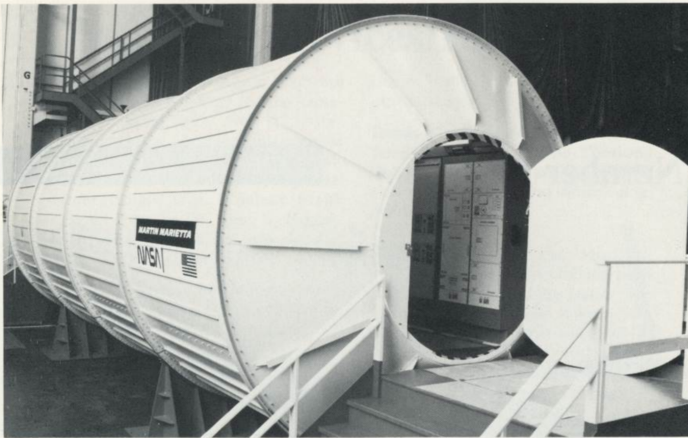
Martin Marietta constructed this full-scale functional model of a space station module at NASA's Marshall Space Flight Center. The company is using the Core Module Integration Simulator to develop technologies and test various systems for the station.
