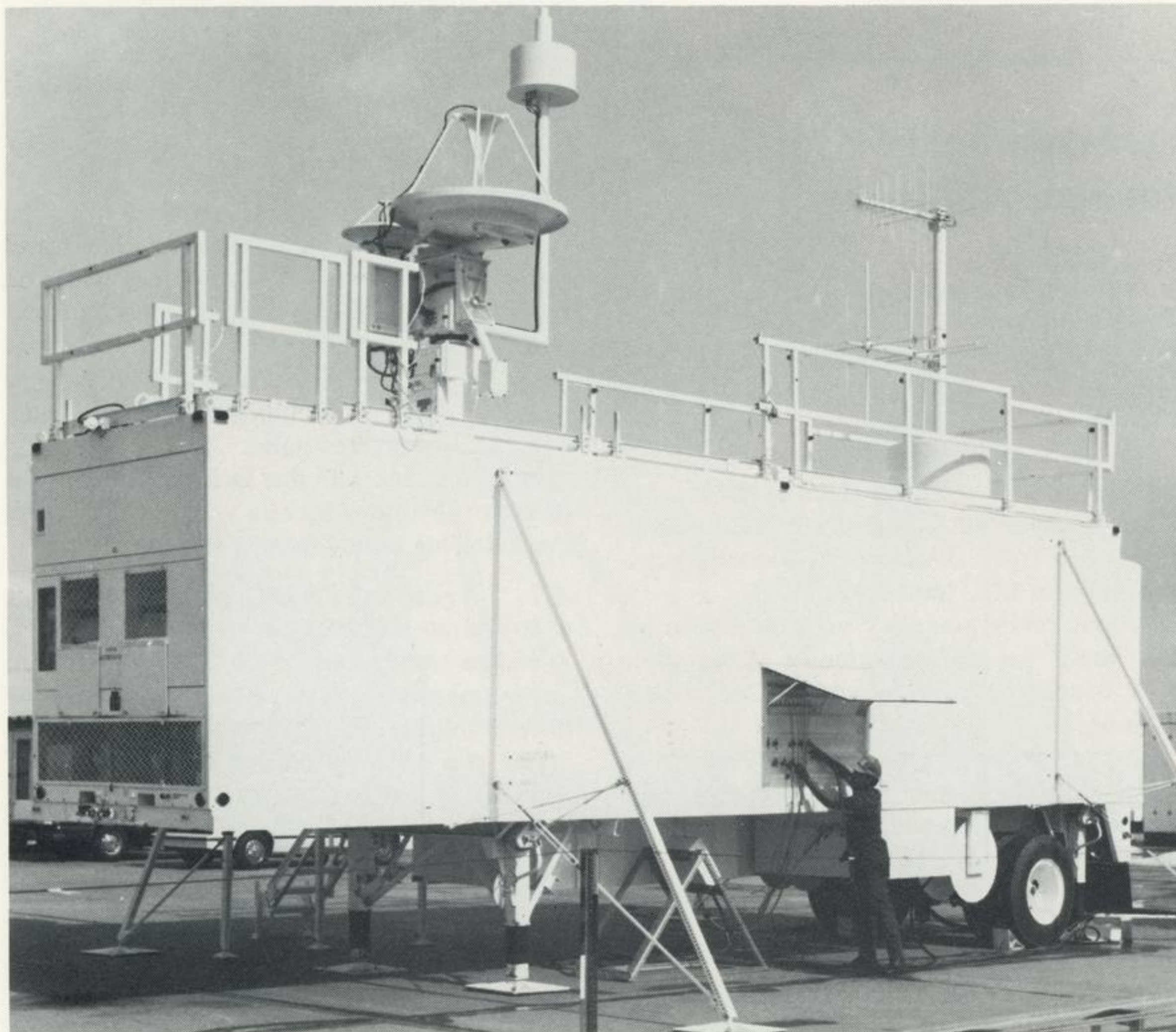
AN/MSR-T4 mobile van is tested before delivery to the Air Force.
