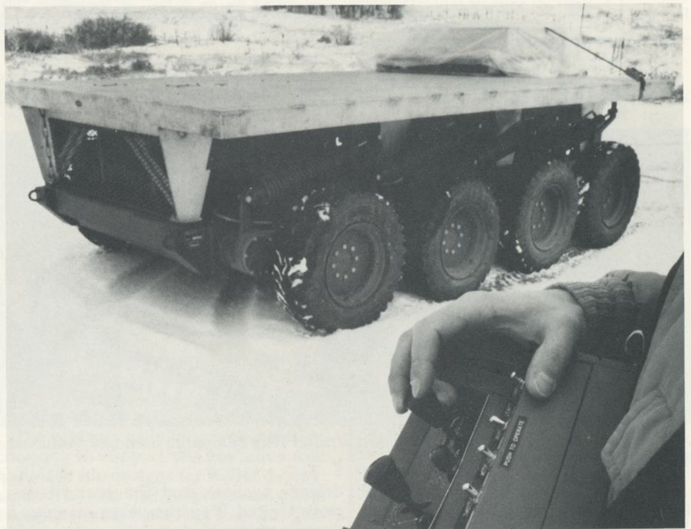
Robot vehicle tested —The 8-wheel base for the autonomous land vehicle is demonstrated at the Waterton plant. The vehicle will be used to show advanced technologies for the strategic computing program—evaluating software, intelligent planners, and advanced computer architecture. May 1985 is the planned milestone demonstration date.
