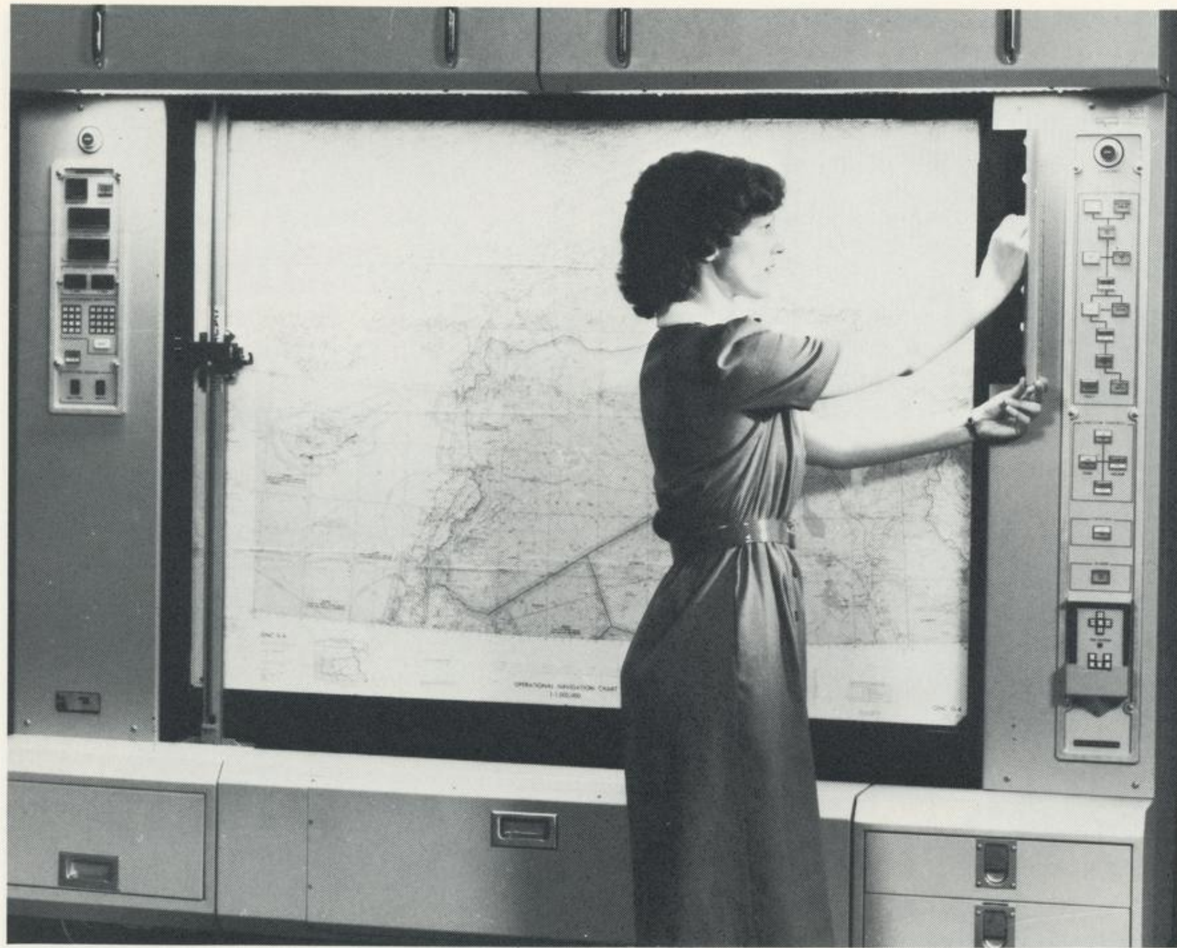
Judy Baity of I&CS adjusts a map on a prototype of a computer-driven plotting system that the company will build for the U.S. Navy. Computer-generated data is mechanically reproduced over standard naval maps by the plotting system.
