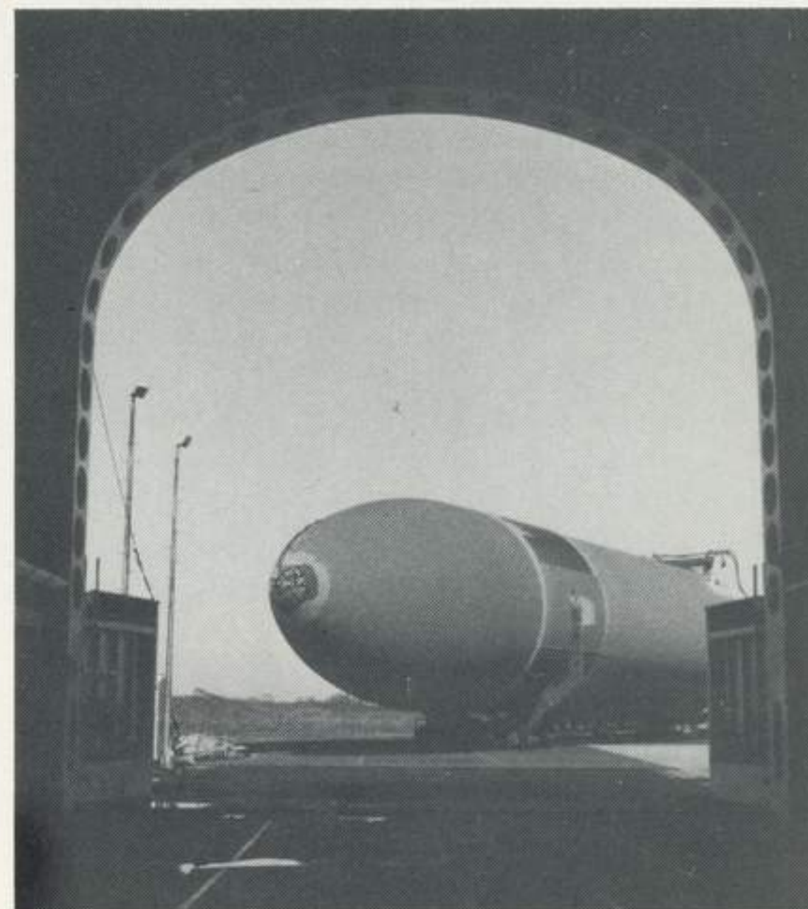
The external fuel tank en route to barge for shipping to Cape Kennedy and ultimate mating with the space shuttle.
