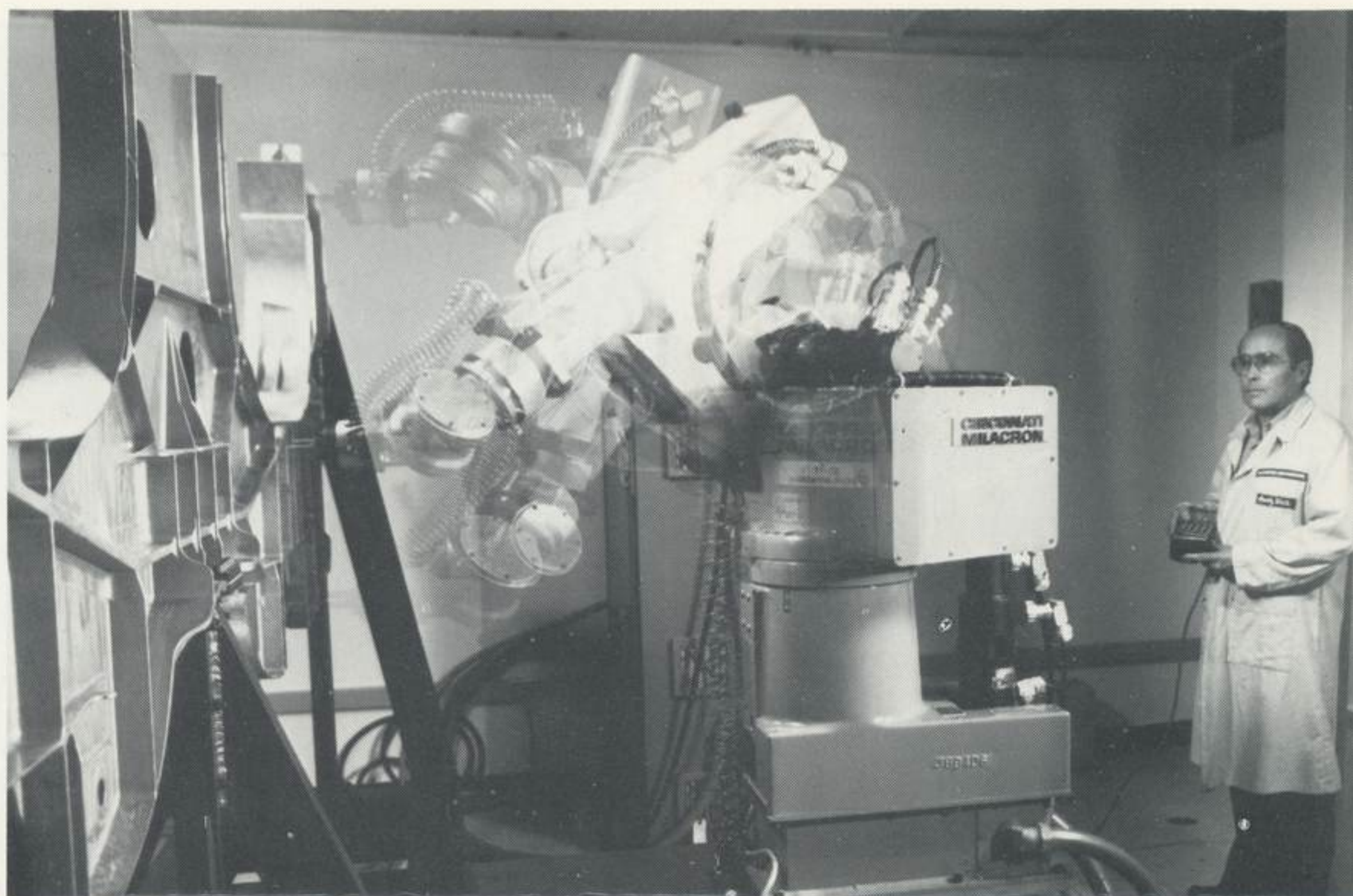
This timed multiple exposure shows a robotic arm in various phases of checking out an F-15 airplane bulkhead in the robotics laboratory. Gordy White, laboratory supervisor, is at the controls.
