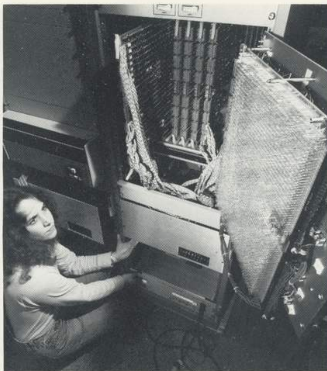
Technician Margie Elkins checks out circuitry on the new PISCES multiprocessor developed for the checkout, control, and monitoring subsystem (CCMS) for the Space Shuttle.
