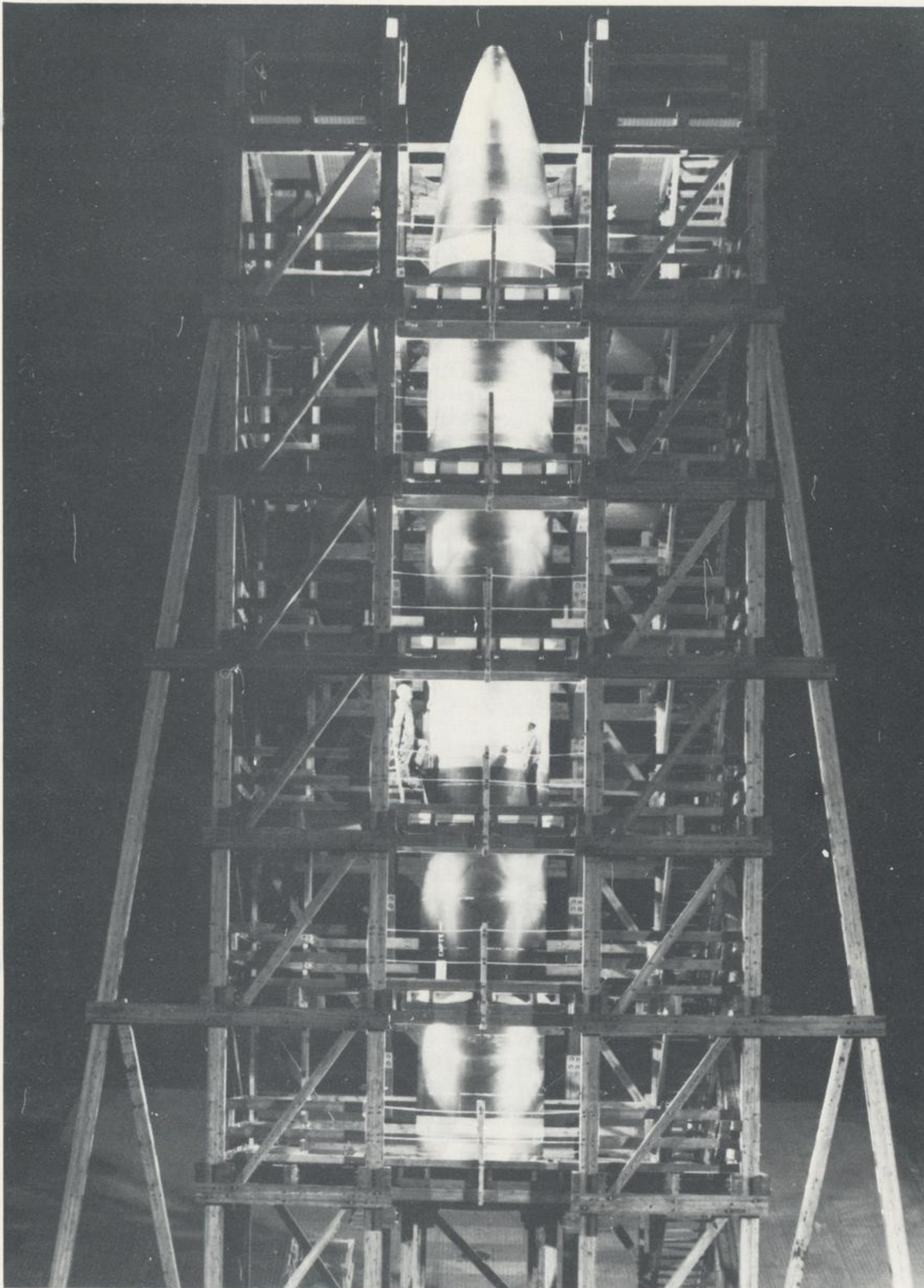
Floodlights illuminate a 71-foot tall Peacekeeper test missile undergoing tests at Defense Nuclear Agency facilities in New Mexico. The tests simulate the electromagnetic pulse generated by a nuclear attack. A wooden structure is used to support the missile, which lacks propellants or warheads, because electrically conductive steel frameworks would influence test data.
