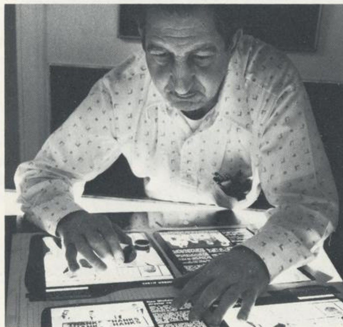
The negatives from which plates are made for the offset press are made and checked by Al Viola in the photo lab.
