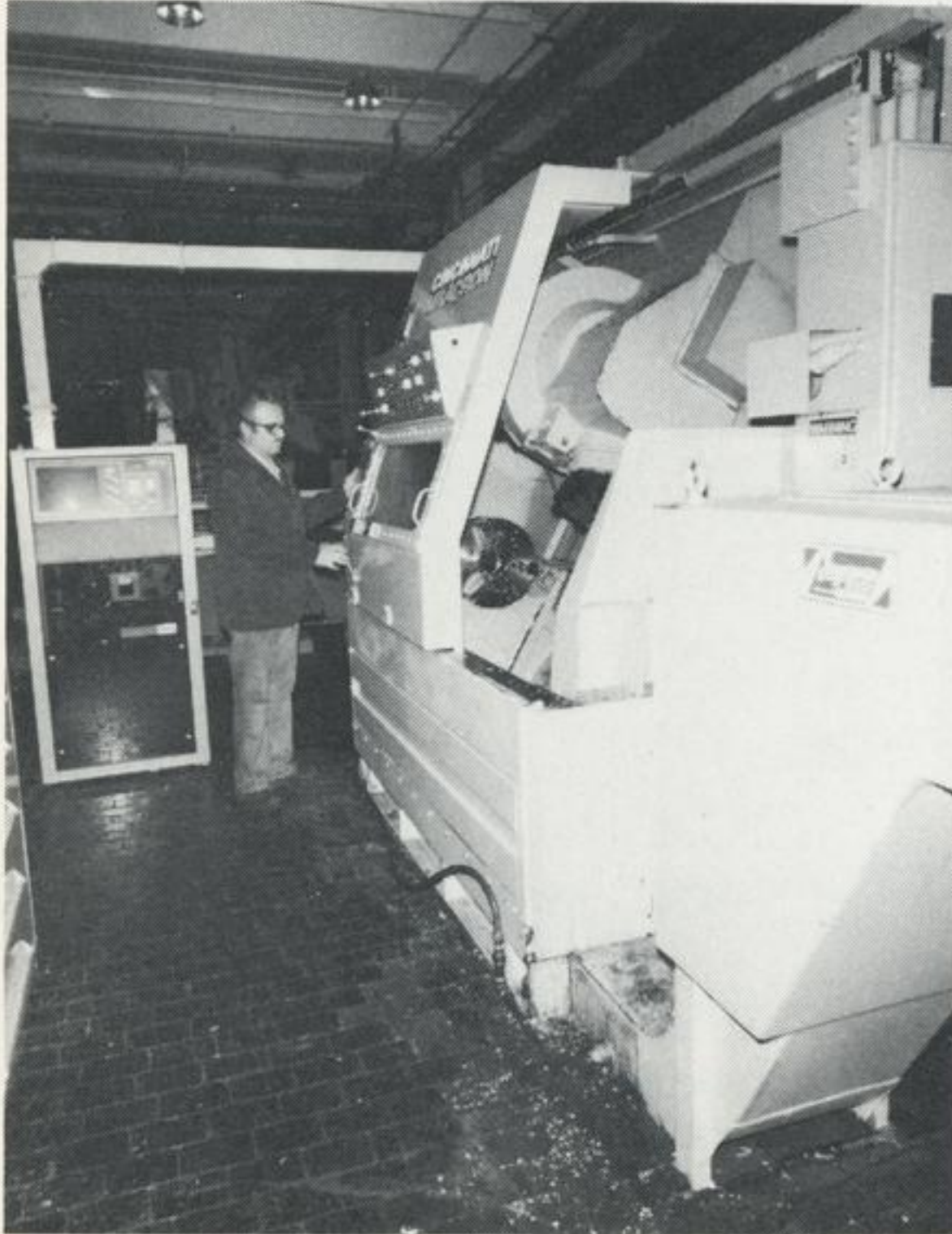
The computer numerically controlled chucker is used by Anthony Globelnik to turn cylindrical-type parts such as Titan pre-valves.
