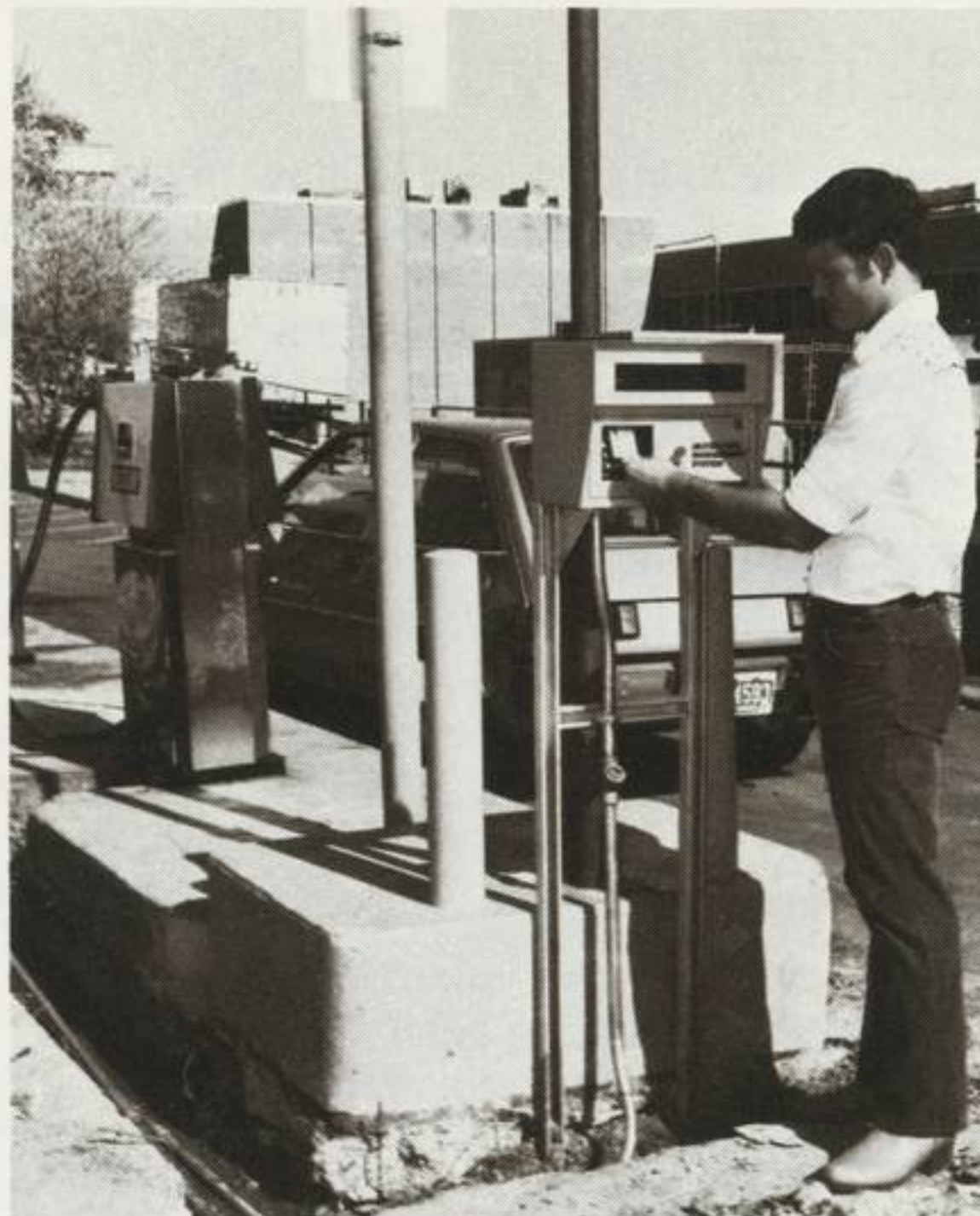
A new motor fuel management system that provides complete vehicle operation records is being demonstrated by systems analyst Kenneth D. LaFreniere.
