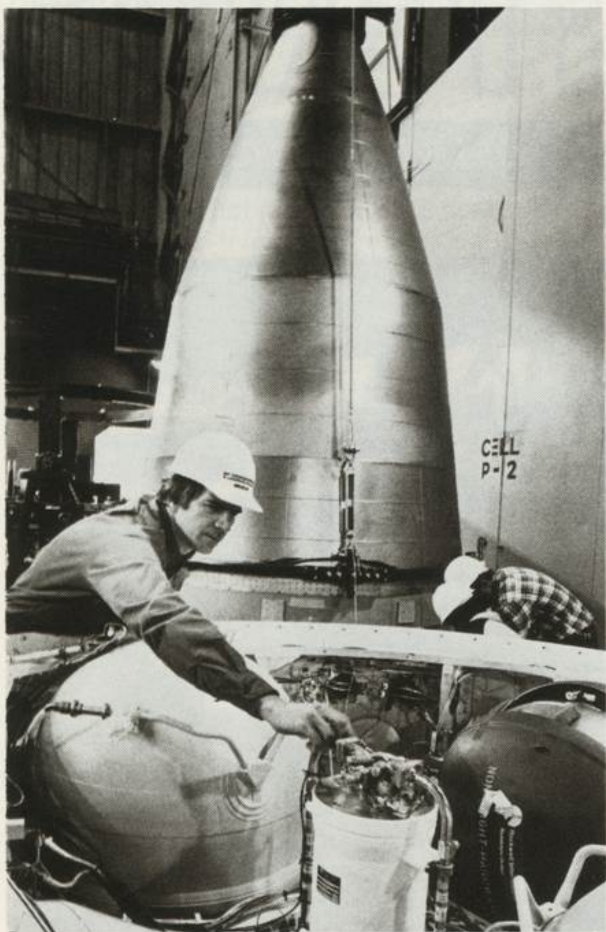
Fourth stage and re-entry system of ground test MX were joined by technicians during the pre-test assembly of a full-size model in the first half of 1982.
