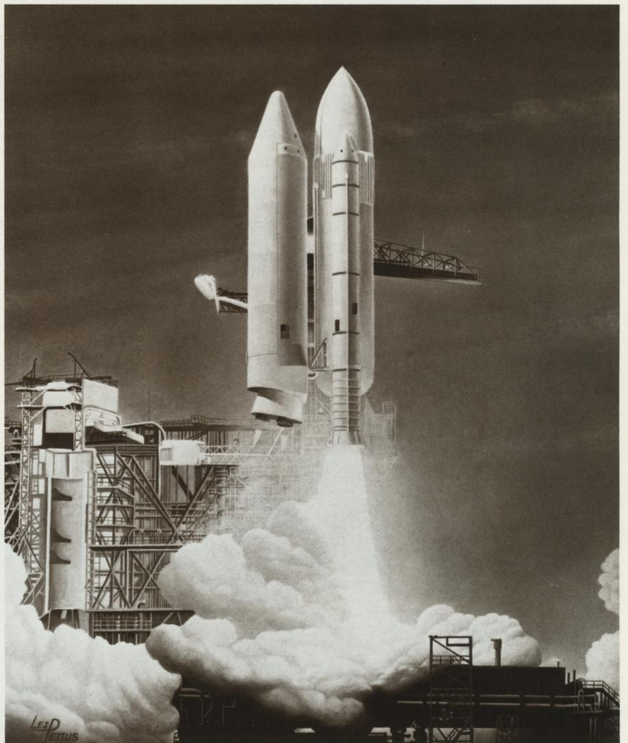
A Shuttle-derived launch vehicle concept developed at the Michoud division lifts off from Kennedy Space Center in this artist's illustration. The launch system depicted here includes an external tank and twin solid rocket boosters like those on the existing Shuttle. The airplane-like orbiter, however, is replaced by a large cargo carrier—an unmanned payload module with reusable avionic and propulsion module incorporating three Space Shuttle main engines. The vehicle would be capable of carrying more than 150,000 pounds of cargo into low earth orbit.
