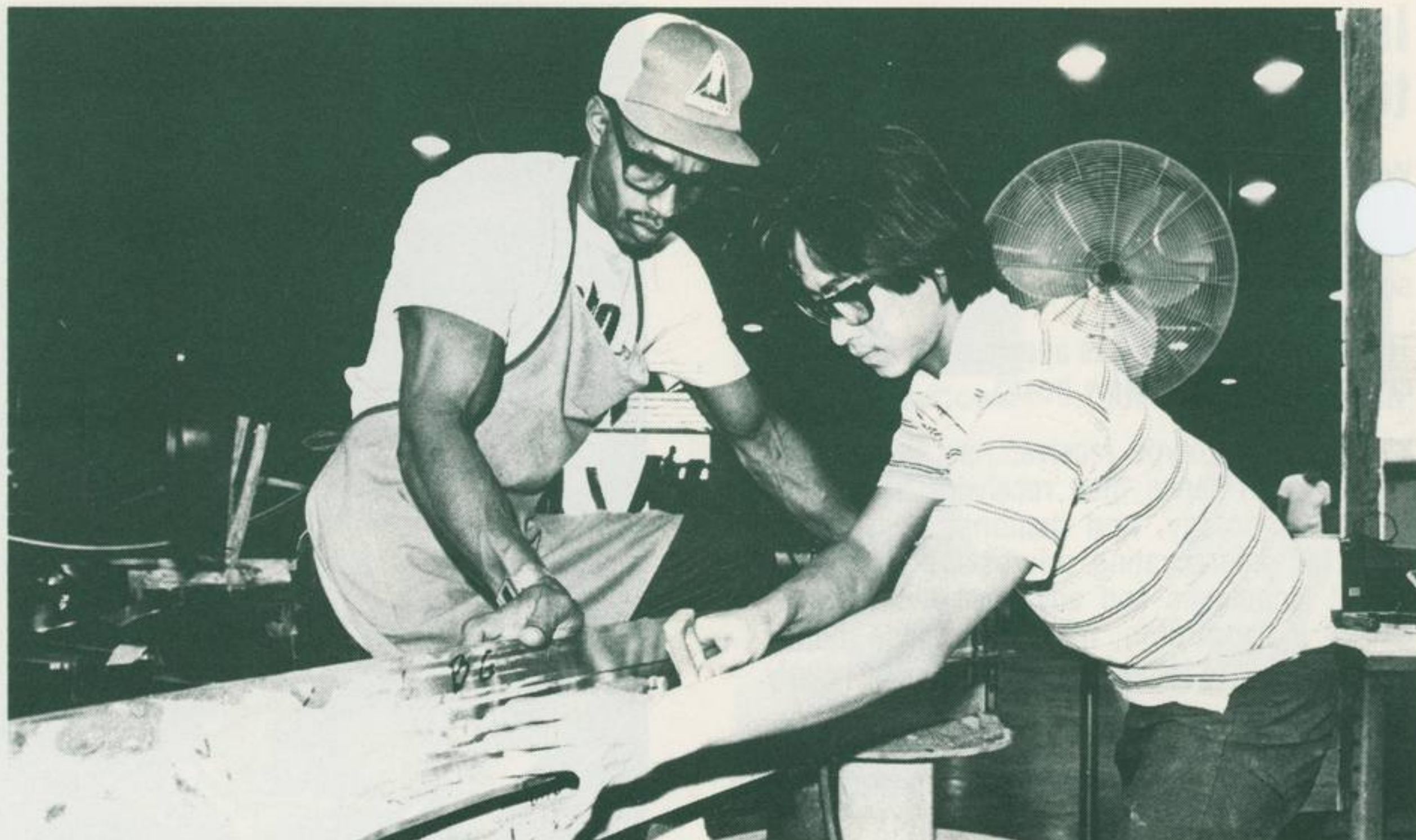
Employees at Aircraft Hydroforming, Inc., inspect a chord section the company machined for the Space Shuttle's external tank. The Gardena, CA company is one of several small firms the Michoud division has subcontracted to make parts for Shuttle tanks. The division was recently cited by NASA for its subcontracting to small and small disadvantaged businesses.
