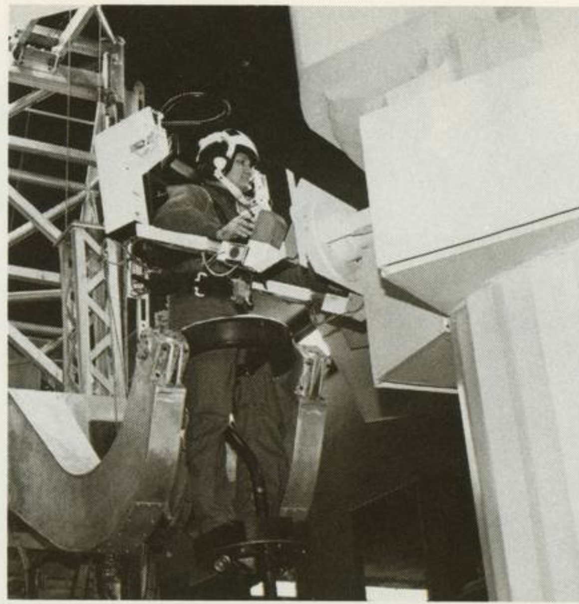
Astronaut Bruce McCandless positions the MMU simulator beside full-scale mockup of a disabled solar mission satellite.
