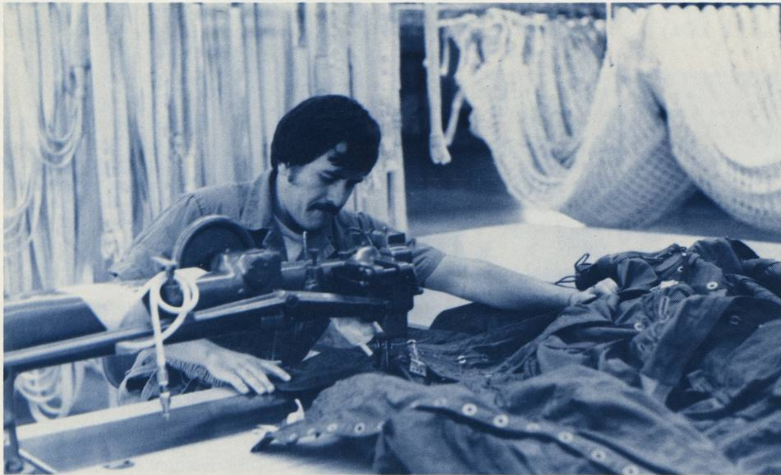
Mark Faucher, a technician for the parachute group at KSC, puts the finishing touches on one of the solid rocket booster main parachute deployment bags. Hanging in the background is one of the drogue parachutes that was recovered after the first Space Shuttle launch.
