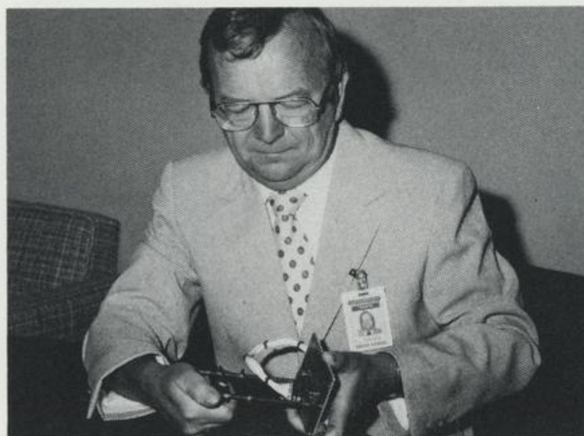
John Turcheck demonstrates the prototype of a demating tool for rectangular connectors. The tool permits greater production efficiency for connector demating.
