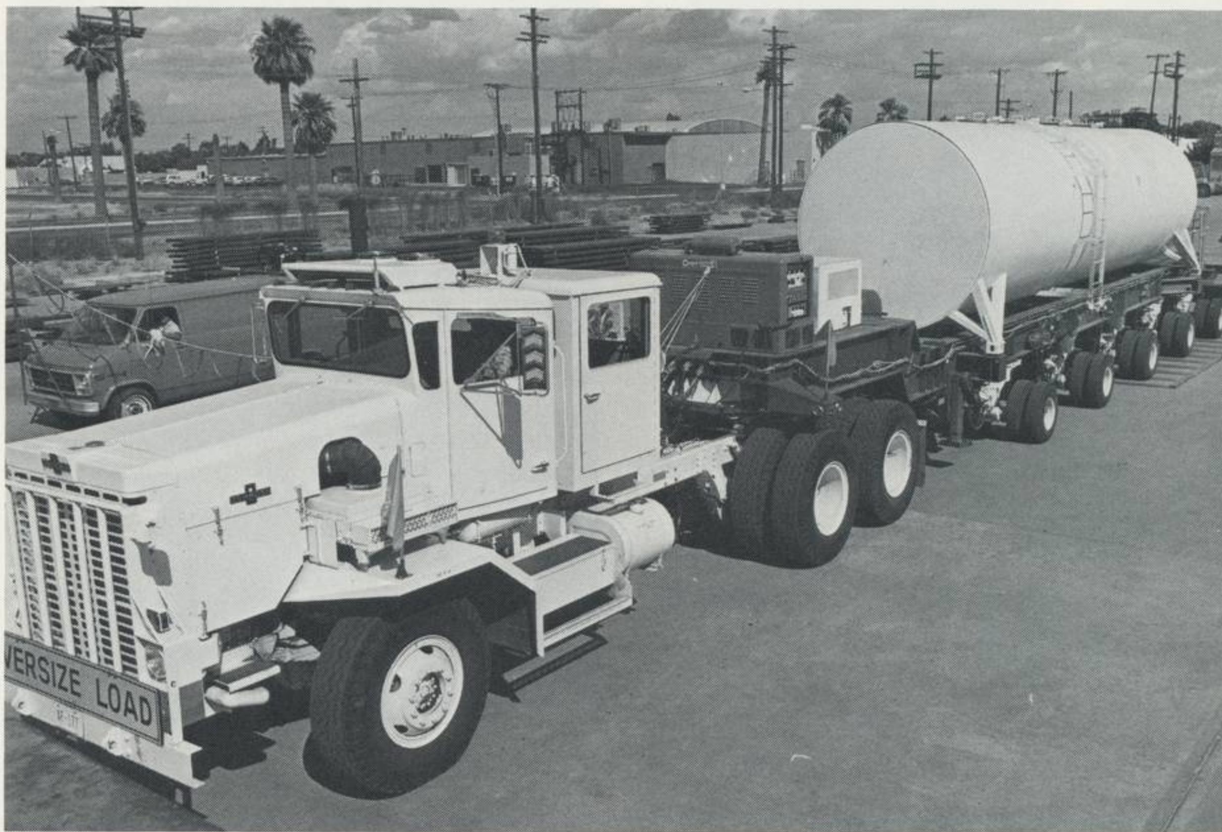
A special 40-wheel tractor-trailer rig has been developed to carry MX missile stages over public highways. The rig, demonstrated recently for the U.S. Air Force, will carry 130,000-pound loads, compared to the 40-50,000-pound loads of the more usual 18-wheeler.
