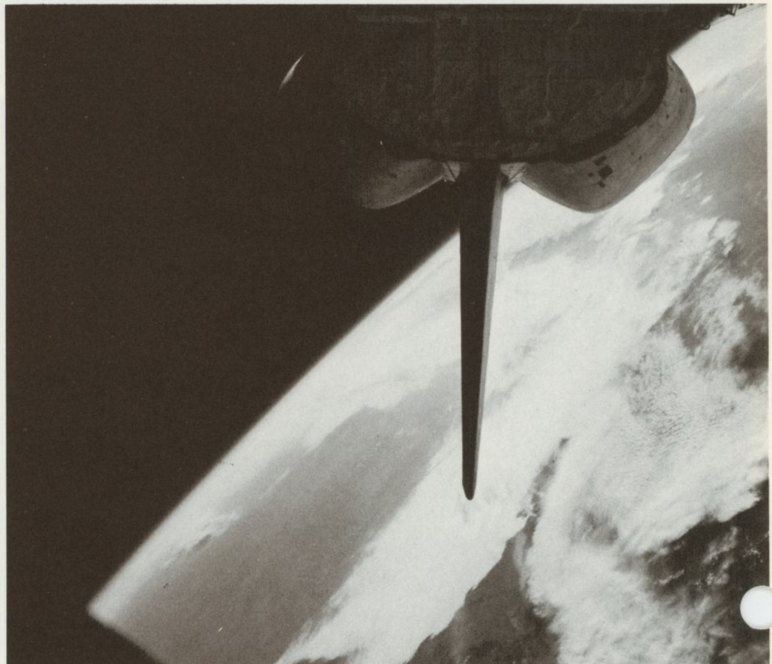
The Earth serves as a backdrop for the silhouetted Columbia's vertical stabilizer and two orbital maneuvering system pods. The photo was taken through aft deck window of the flight deck.
