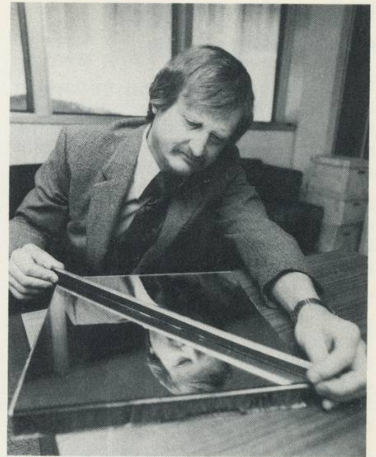
Demonstrating the curvature of his free-floating heliostat mirror assembly invention is Kenneth A. Karki, strategic systems division. The removable mirror is attached to a steel-faced honeycomb assembly by magnets.
