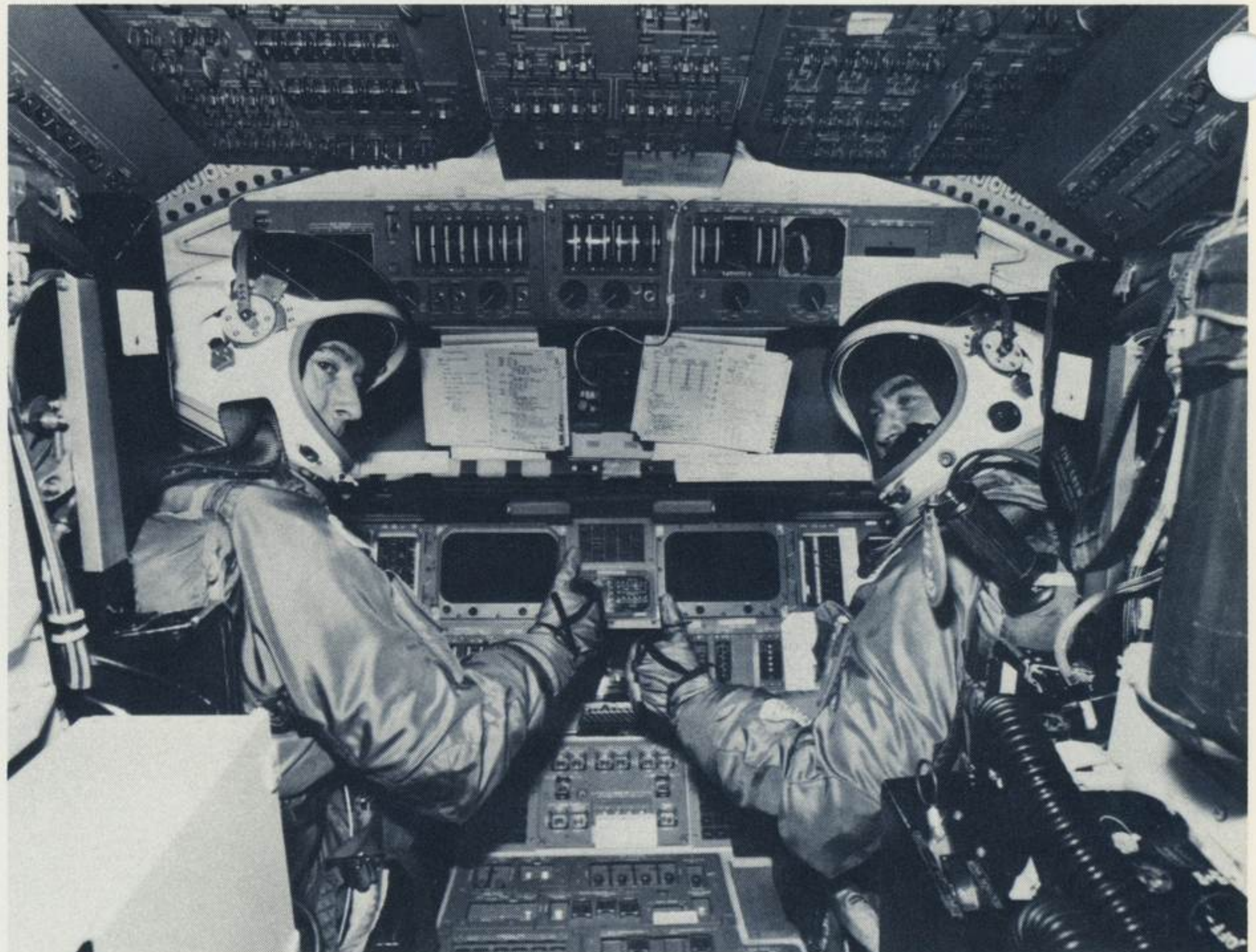
Commander John Young and Pilot Robert Crippen, crew for the first Space Shuttle mission, took a break from training to pose for this photo on the flight deck of the orbiter Columbia. Shown are the TV-like displays, and duplicate sets of hand controllers, pedals, levers, and switches with which either astronaut can fly the craft alone. The astronauts are wearing ejection escape suits that will be worn only during the orbital flight test program and then only during the launch and landing phases of the mission.
