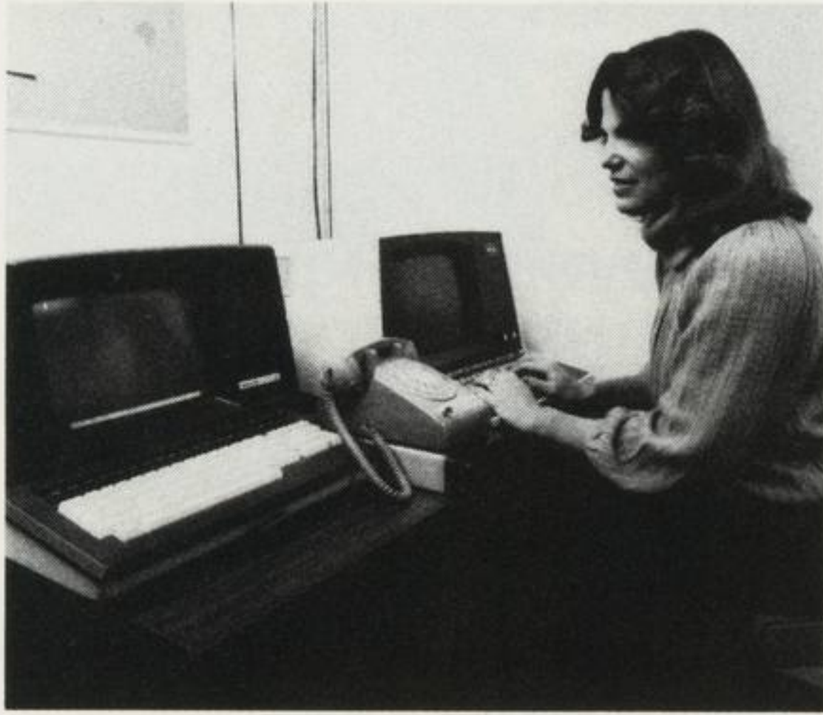
Two electronic mail terminals can be operated by Paula Curra at this station in the evaluation that begins in April. Messages travel from station to station over normal telephone lines.
