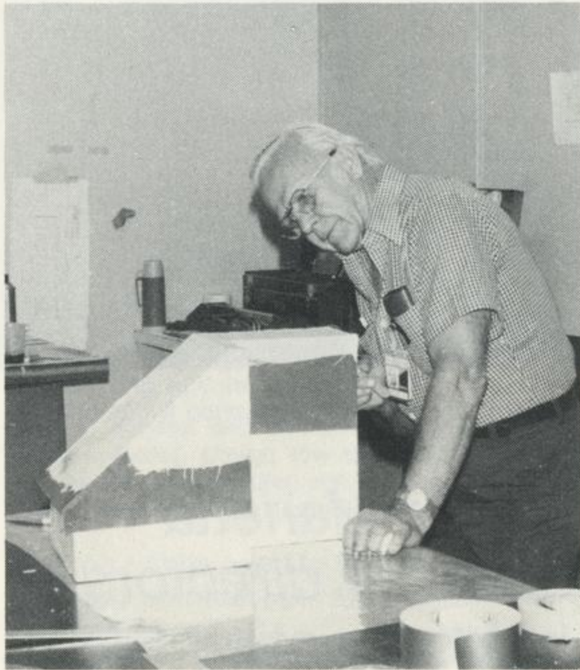
Epoxy is spread on a styrofoam form before fiberglass cloth is applied to build a mold for external tank modification. Fred Burlew is preparing the mold.
