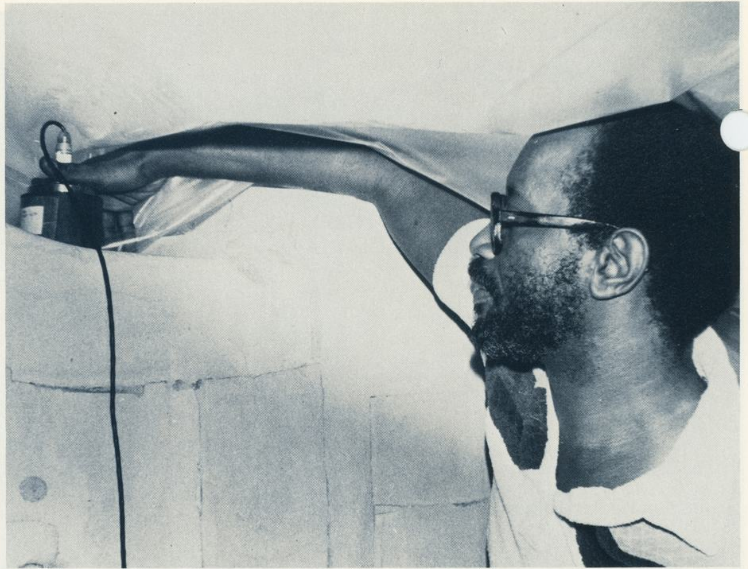
Taking a Kaman reading on a vertical strut on the first flight external tank at Kennedy Space Center is Charles Owens, a Michoud division technician on temporary duty at the division's external tank operations at KSC. The meter is used to electrically measure the thickness of the thermal protection system (TPS). The thickness varies depending on the area of the external tank and must meet strict design standards.
