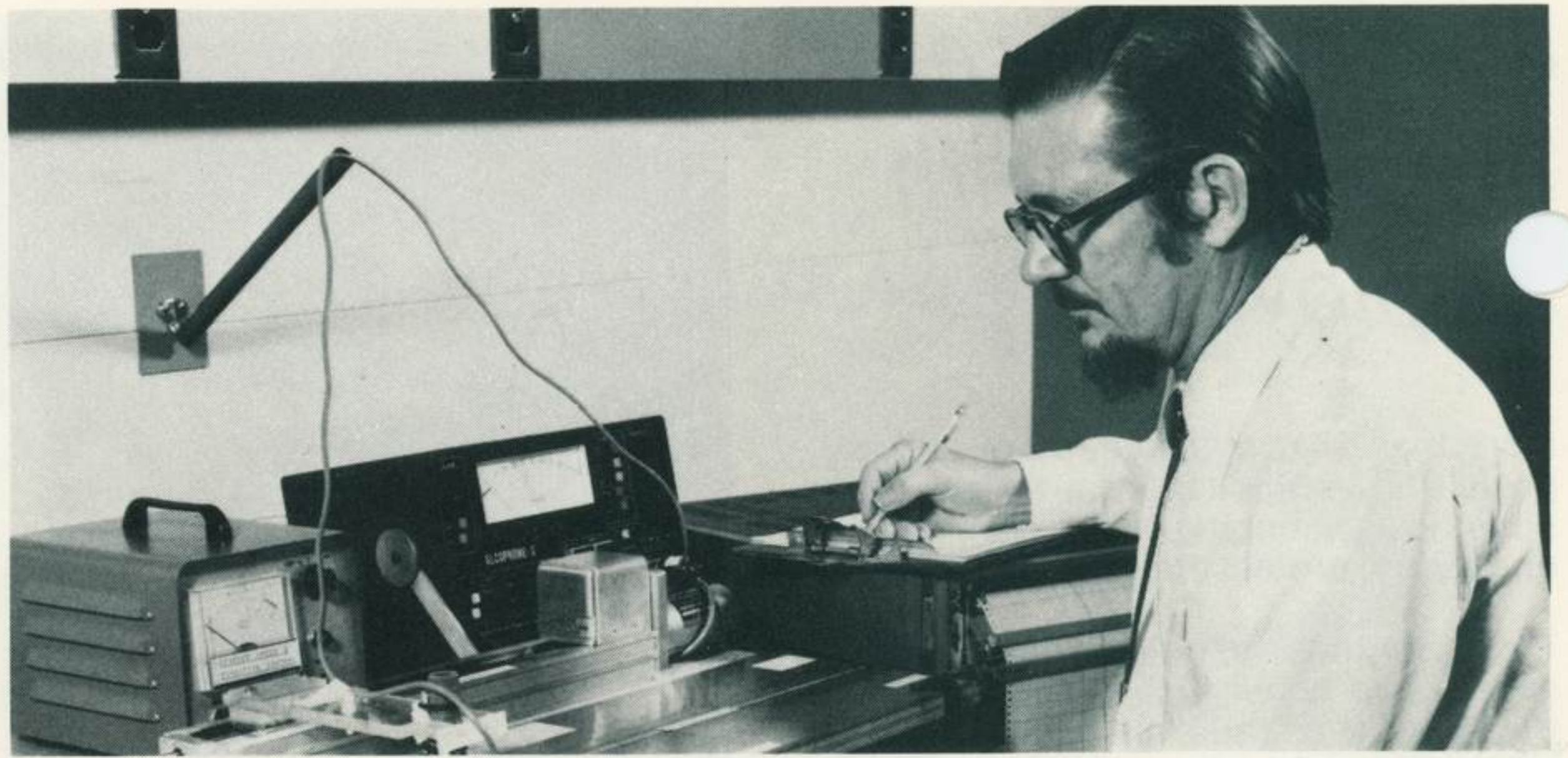
Michoud division group engineer James B. Beal evaluates deep eddy current equipment on a typical external tank tapered thickness weld.
