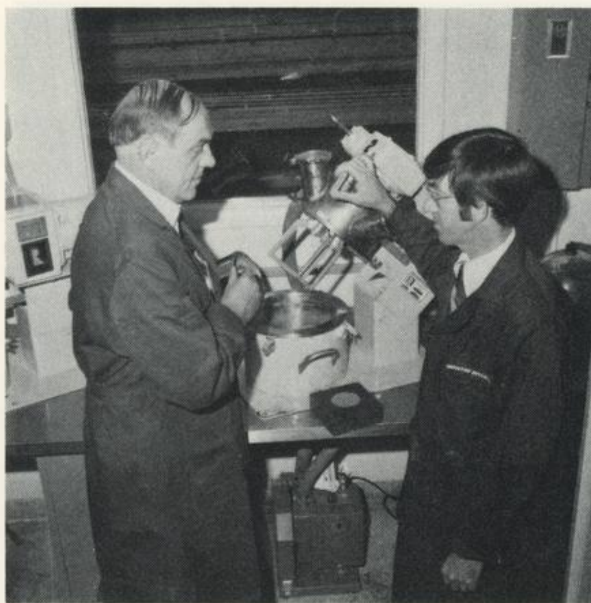
Ronald W. Graese, left, and Ronnie L. Campbell, right, are shown mixing a modified ablator material that may be used for in-flight repair of Space Shuttle ceramic tile. The men have received a new technology award for their work on the modification.
