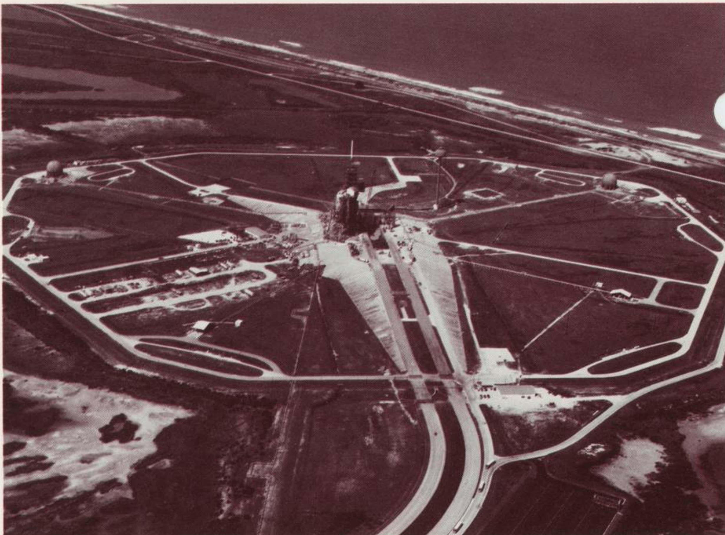
In this aerial view of launch complex 29, pad A, at Kennedy Space Center, the liquid oxygen storage is shown at the upper left and liquid hydrogen storage at upper right. Lines from these areas supply propellants to spacecraft at the center of the complex.
