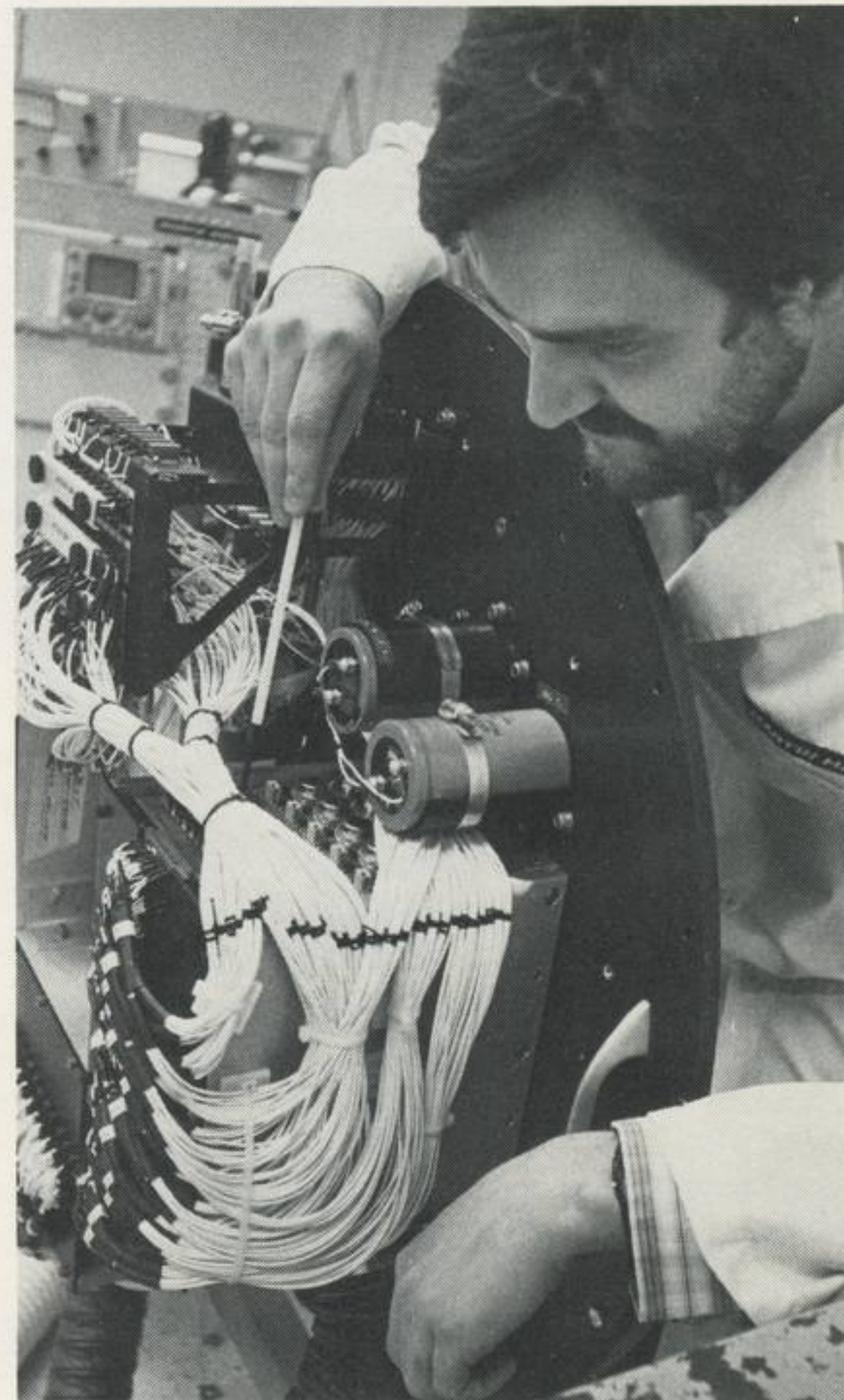
This electronic imaging device, attached to a large telescope in a high-altitude aircraft, will gather data on the heating of Shuttle orbiter's insulation tiles during re-entry. Electrical engineer Roy Sebring adjusts the instrument before it was shipped.
