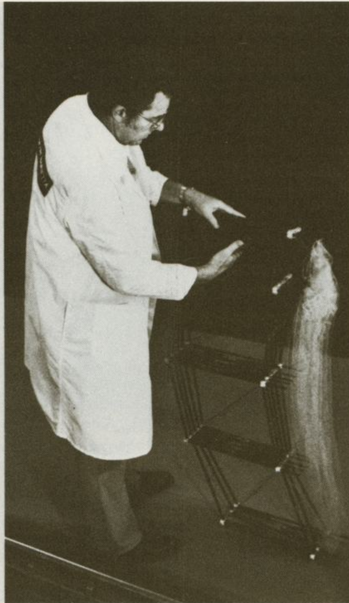
Senior engineer William H. Tobey is shown deploying a scale model antenna. At left, the structure is in the stowed position; in the center, deployment is begun; and at right, the model antenna is fully deployed. In space, the antenna could be up to 600 feet wide.
