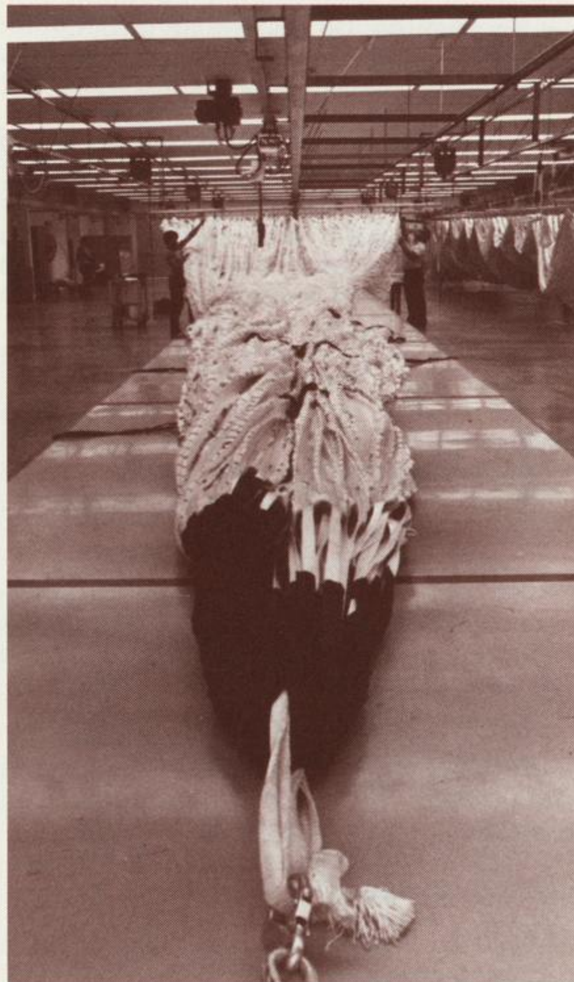
One of the three main parachutes to be used for recovery of the Space Shuttle solid rocket booster is shown in this NASA photo as it was being packed at Cape Canaveral. The parachute measures 230 feet from the top to the ends of the suspension lines. It weighs 1,700 pounds.
