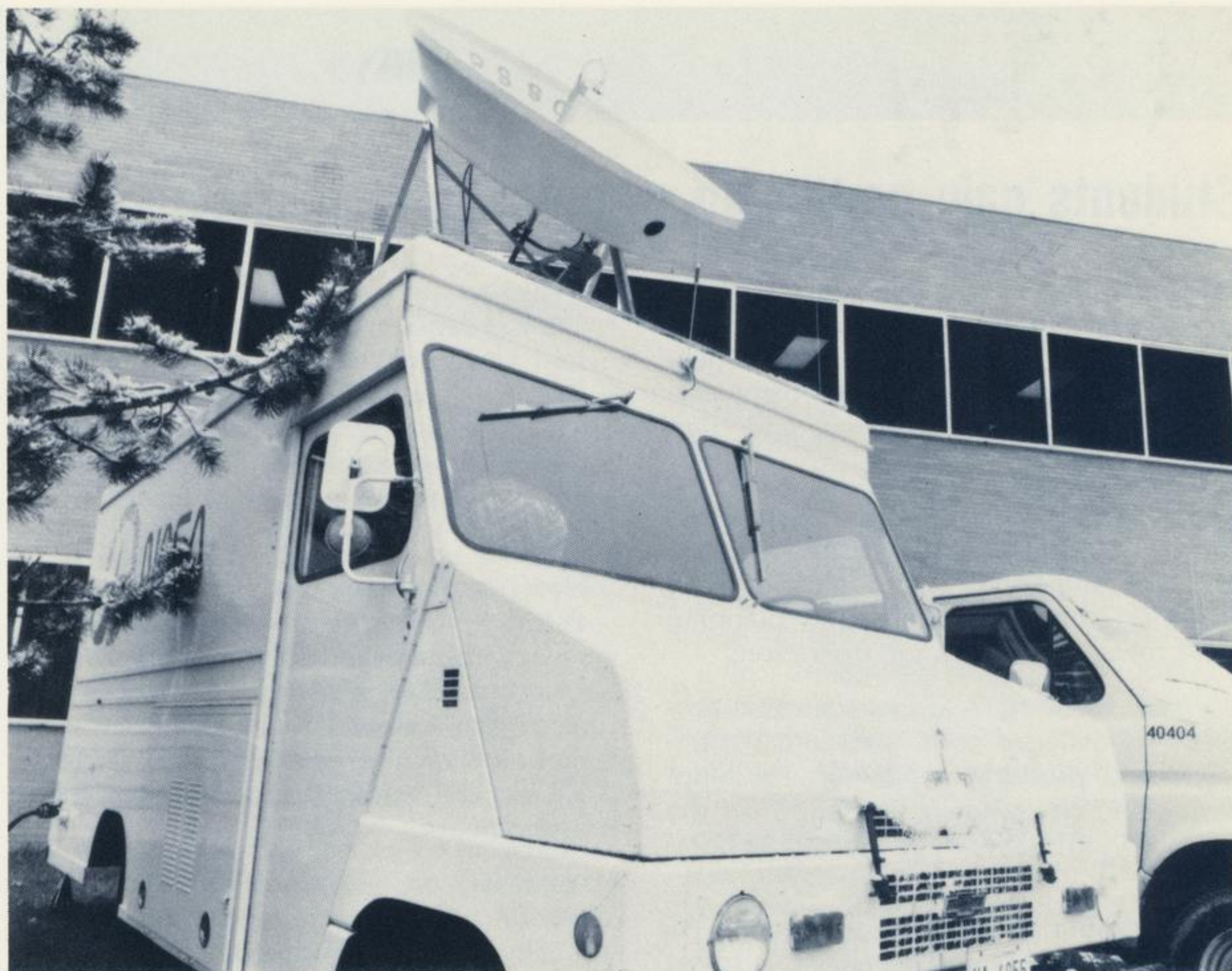
Public Service Satellite Consortium van contained transmitting and receiving equipment for the two-way satellite communications for the critical design review.
