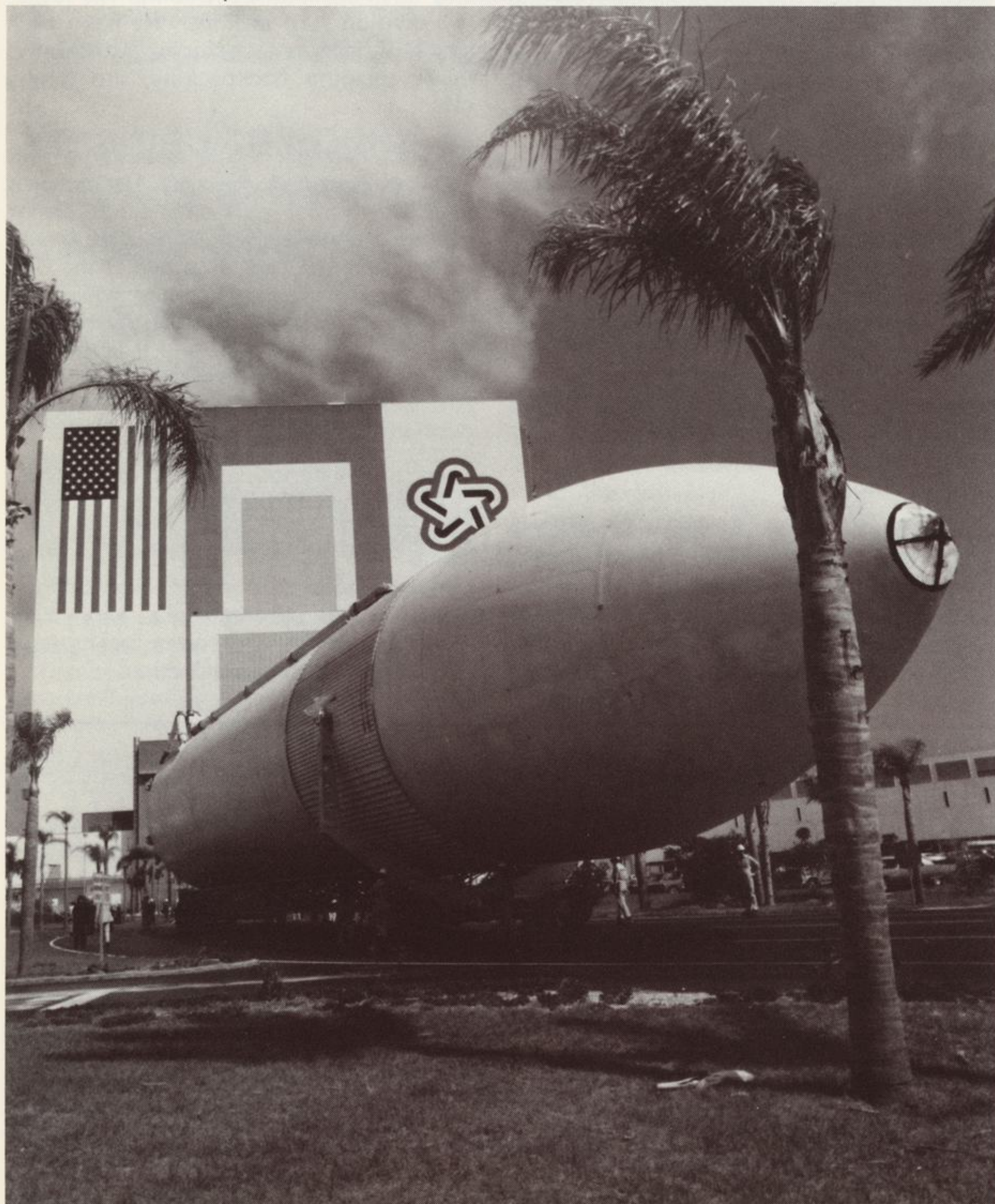
The first Space Shuttle external tank delivered to Kennedy Space Center was recently moved to the vehicle assembly building. The tank is not a flight version but is a ground vibration test article used at Marshall Space Flight Center.
