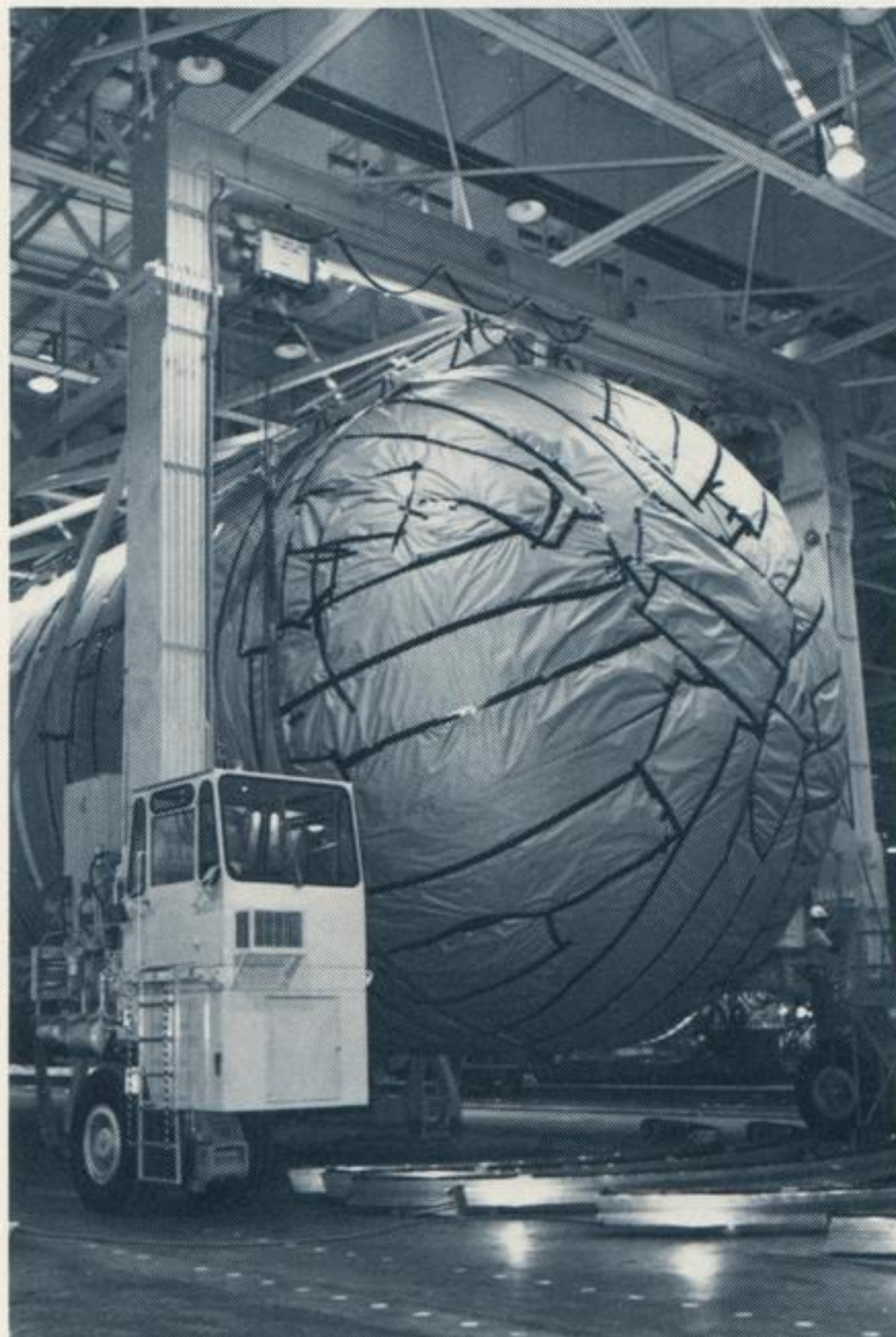
A huge straddle carrier transports the hydrogen tank portion of flight external tank number 2 to a pneumastatic test facility for pressure tests. The tank is wrapped in heavy brown paper to protect it from contamination in the air before installation of the foam-like thermal protection system coating.
