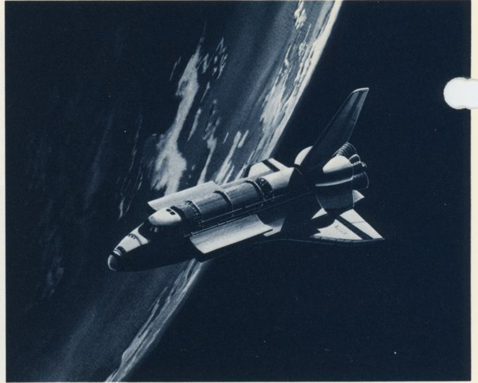
The orbiter payload shown in the cargo bay consists of the array structure and a low thrust liquid transfer stage.
