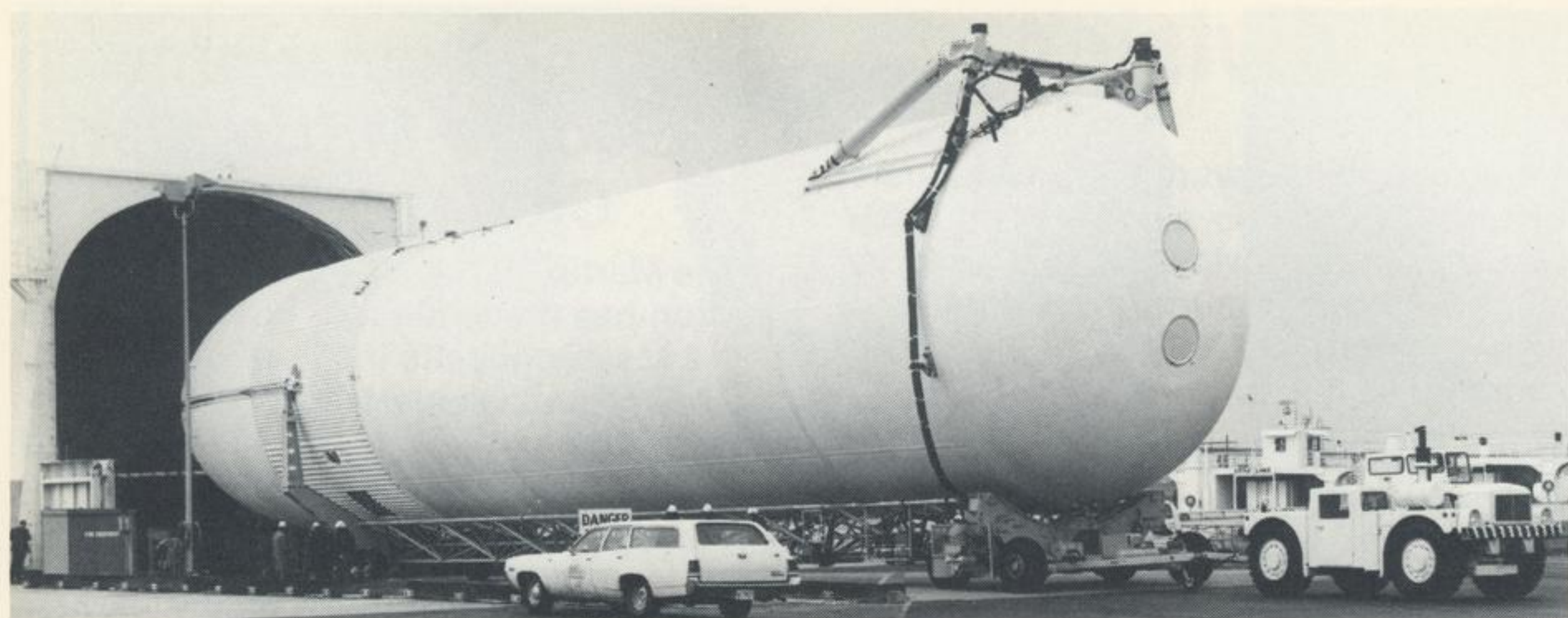
A completed Space Shuttle external fuel tank is loaded on its covered barge at Port Michoud in preparation for an 11-day journey on the Mississippi, Ohio and Tennessee Rivers to Huntsville, Alabama.
