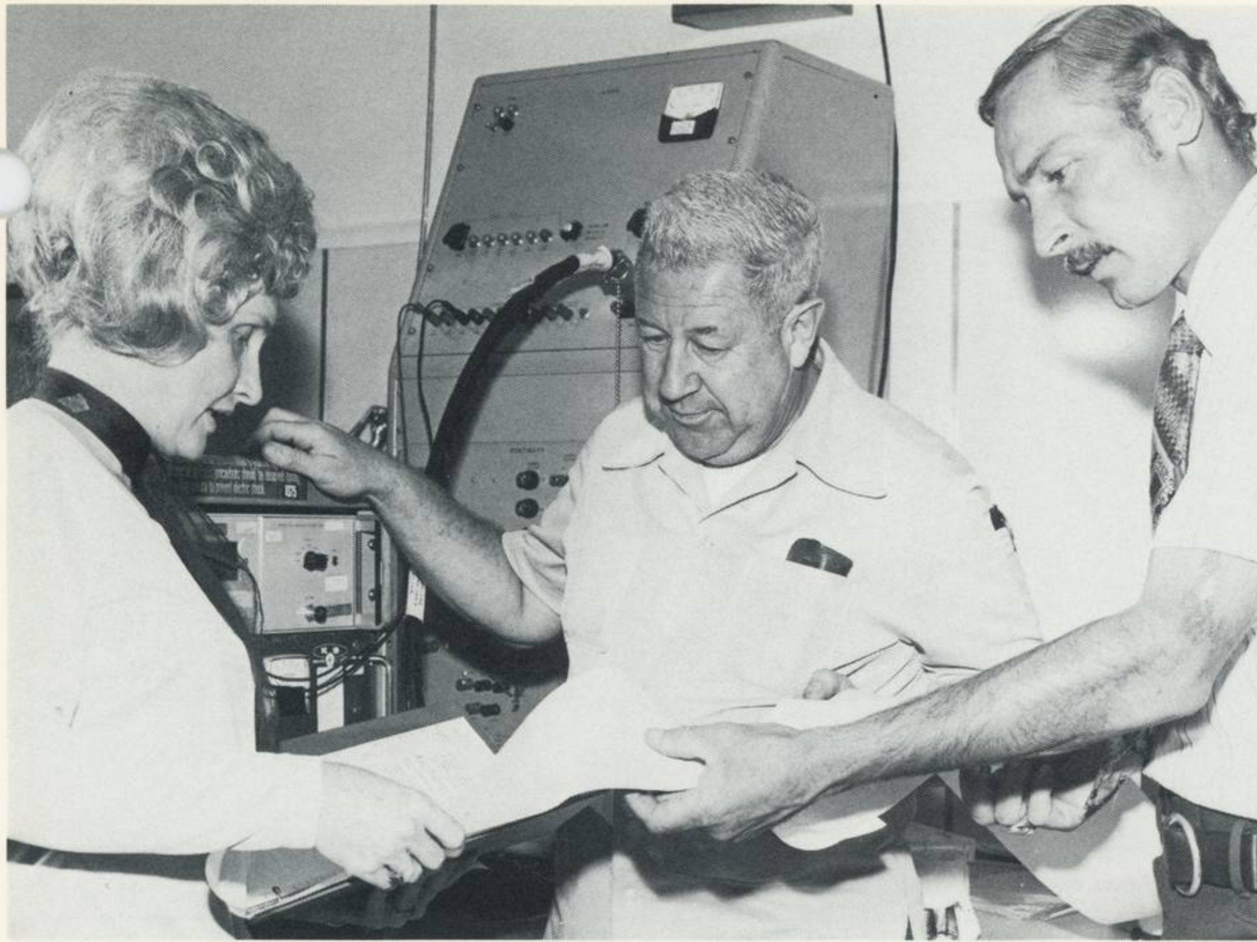
Elinor Durso and Bill Hunt, CMA Supervisor, with electrical technician Dick Guay, check voltage and current recorder reading of an airborne flight battery.
