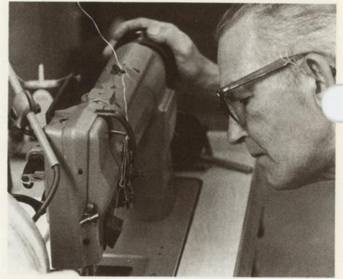
Ford Cassel uses a high-speed, factory-type sewing machine to replace worn SCAPE suit zippers as part of the maintenance program for the ensemble. Cassel, a mechanical technician, has been at Vandenberg since 1959.
