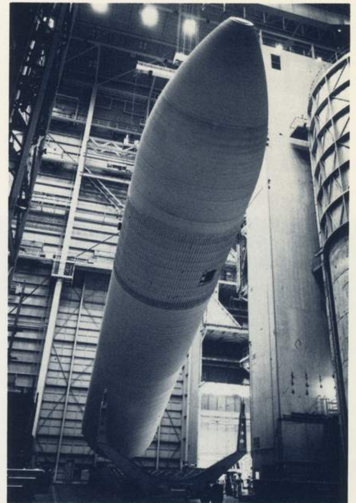
Completed external tank is lowered from a vertical position to the transporter that will carry it to a barge on the Pearl River.
