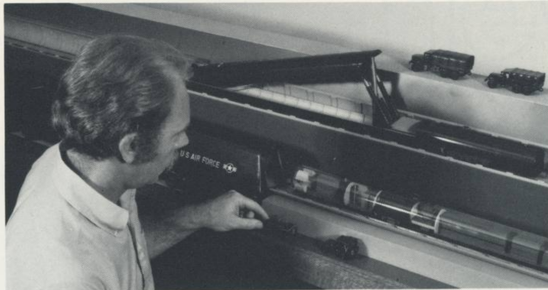
D. J. Hughes, program planner, arranges model of buried trench weapon system showing, from top to bottom, the transporter/launcher with canister elevated, the mobile launch control center, and transporter.
