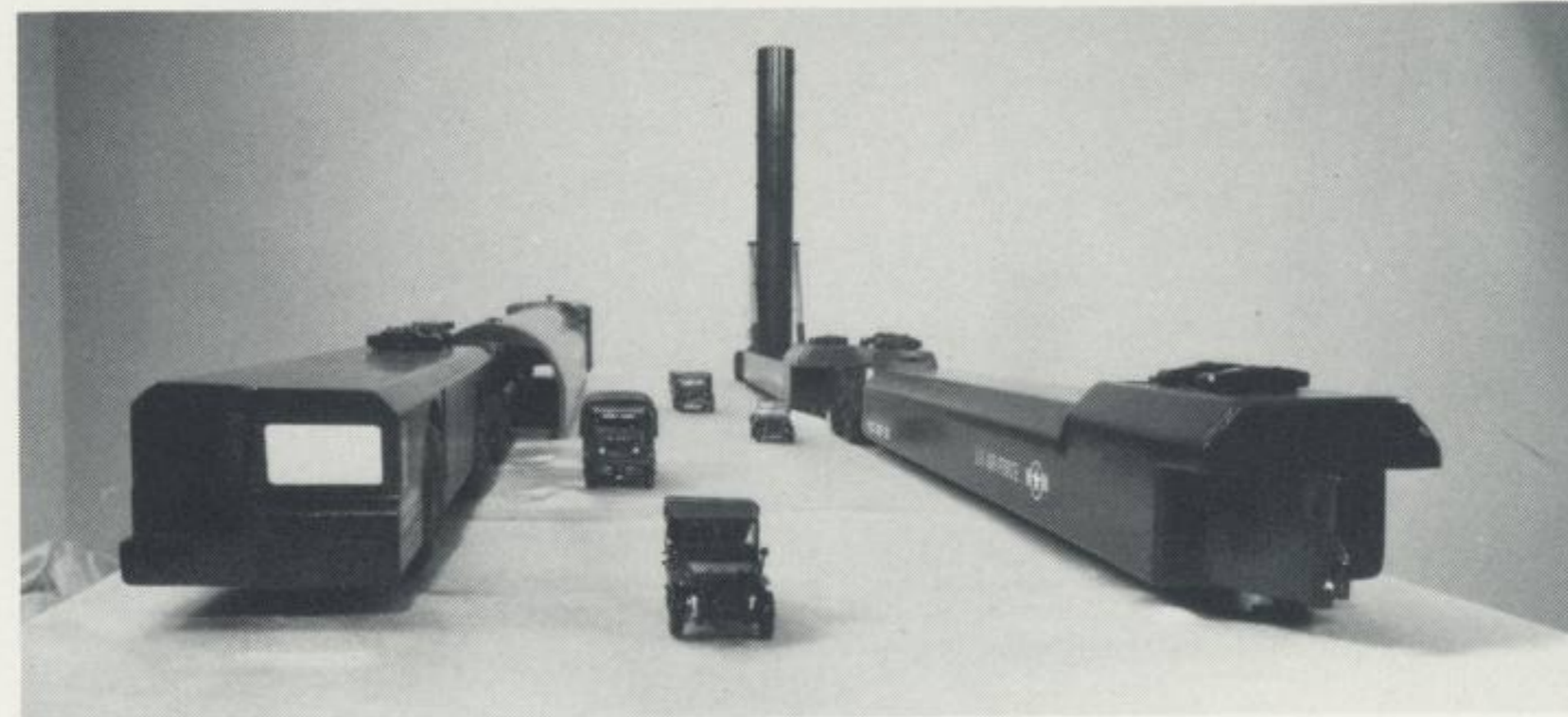
Phase one study for MX produced concepts for above ground vehicles for a shelter-based weapons system. The models depict the vehicle transport, mobile launch control center, and the missile launch vehicle with the missile canister in launch position.
