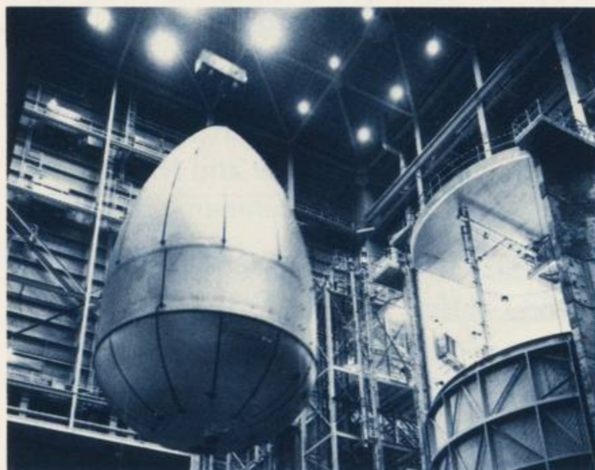
Liquid oxygen tank is moved by straddle to the vehicle assembly building (top) and then lifted into the hydrostatic test cell (bottom).
