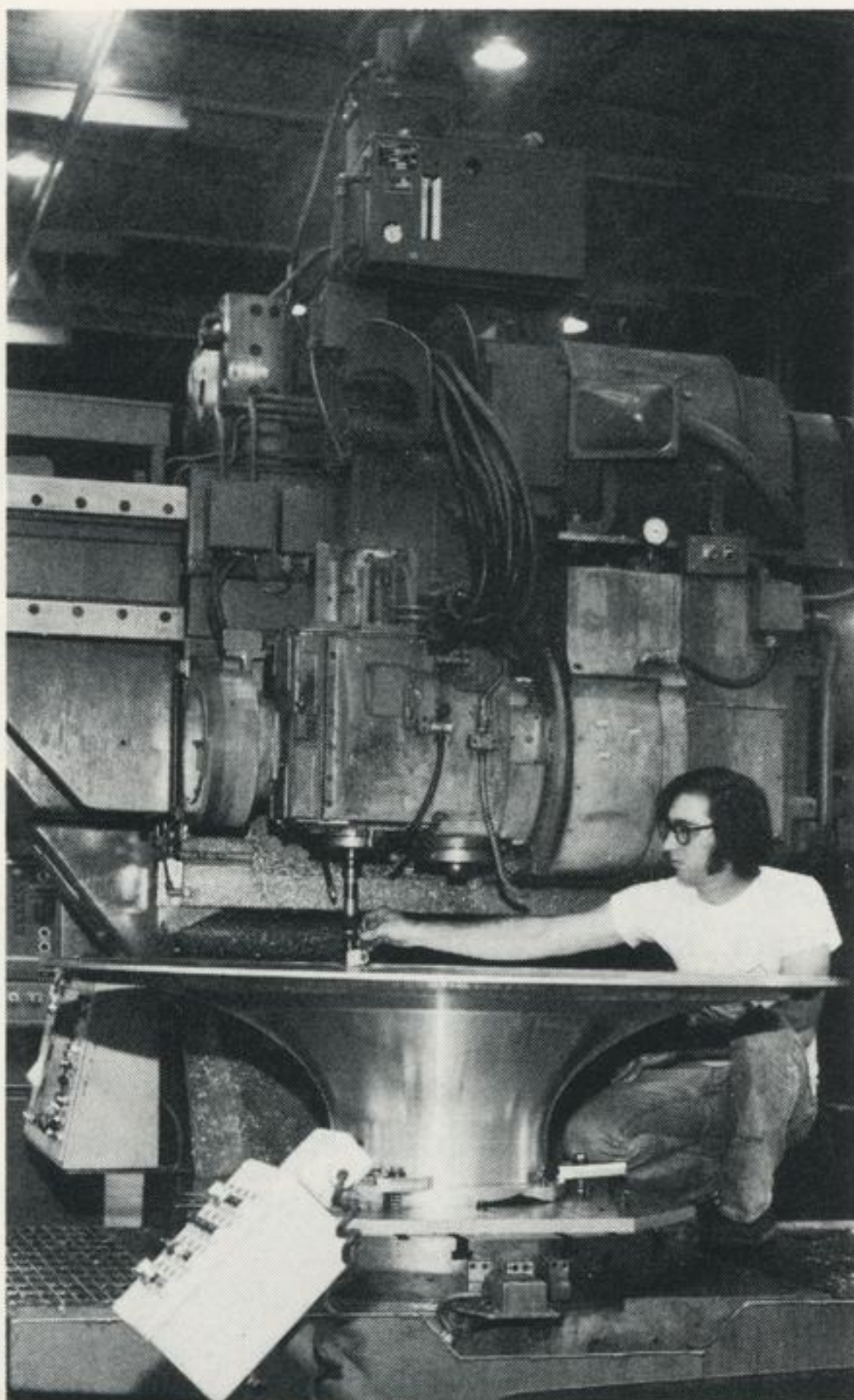
Machinist James Matthews adjusts a tape-controlled Omnimil before machining a fuel suction fitting that will be welded onto the liquid oxygen tank dome of the external tank. The machine can perform seven different operations from its taped program.
