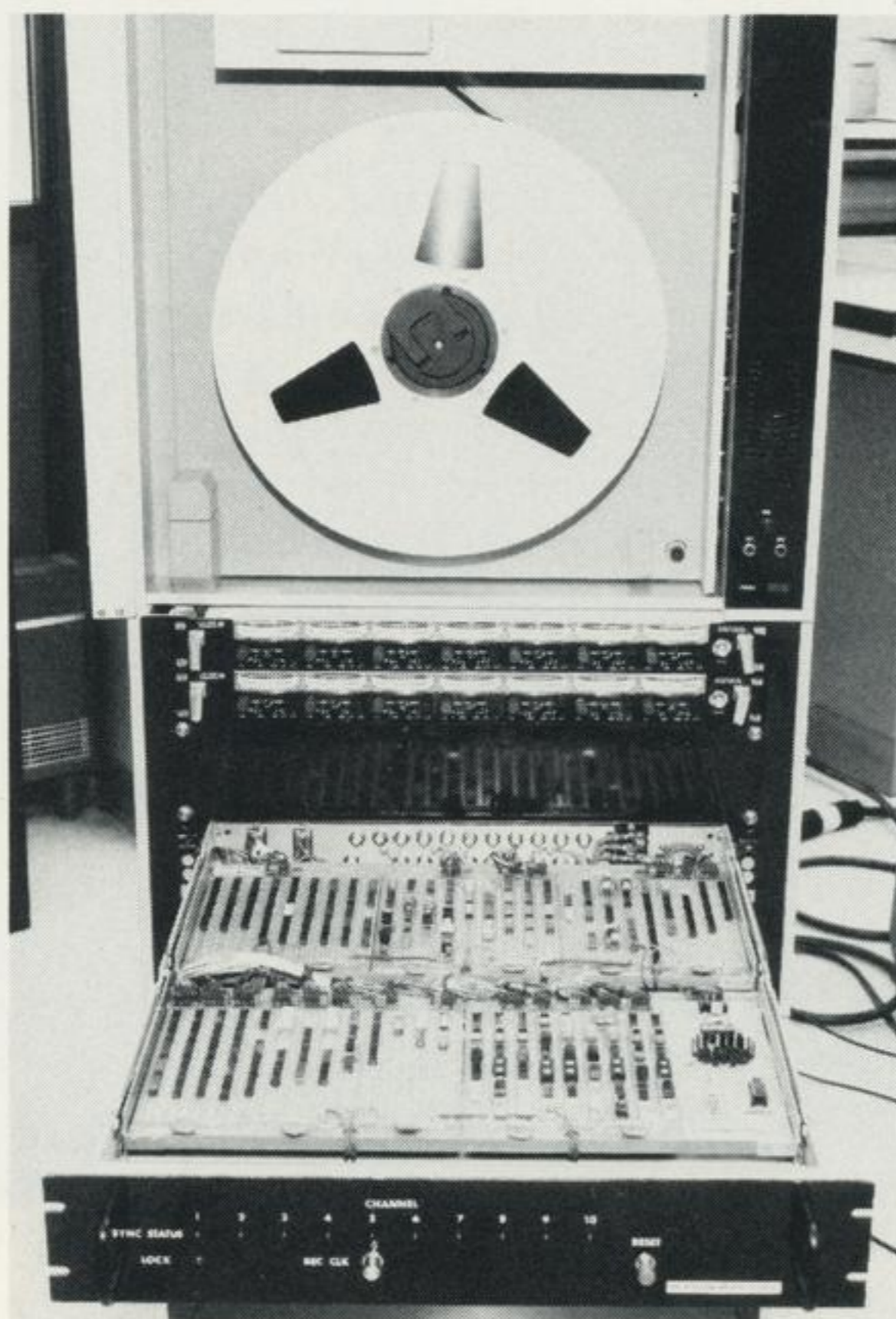
Drawers in tape recorder contain division's hardware for high density, high rate digital data recorder.
