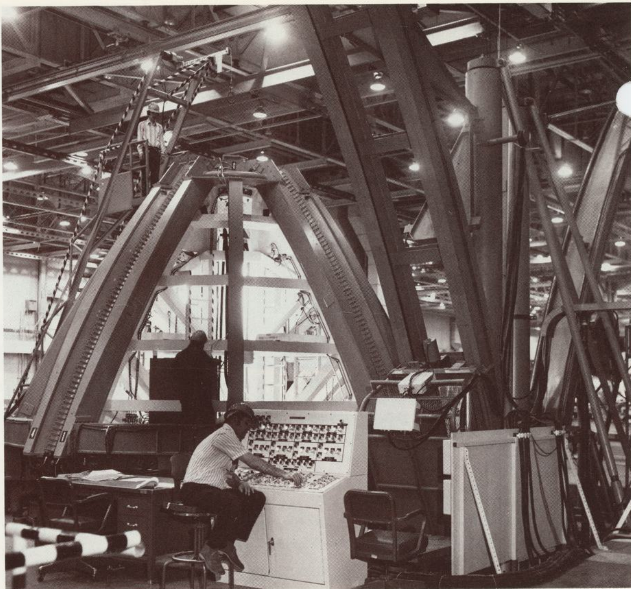
Doug Sharp (at the console), Jay Williams and Ben Jurado (top side) check over the latest addition to Michoud's major production tooling—forward ogive trim and weld fixture. This 130,000 pound fixture, trims and welds together the eight panels and forward closure fitting of the forward og assembly of the external tank. The fixture was designed and fabricated by General Dynamics.
