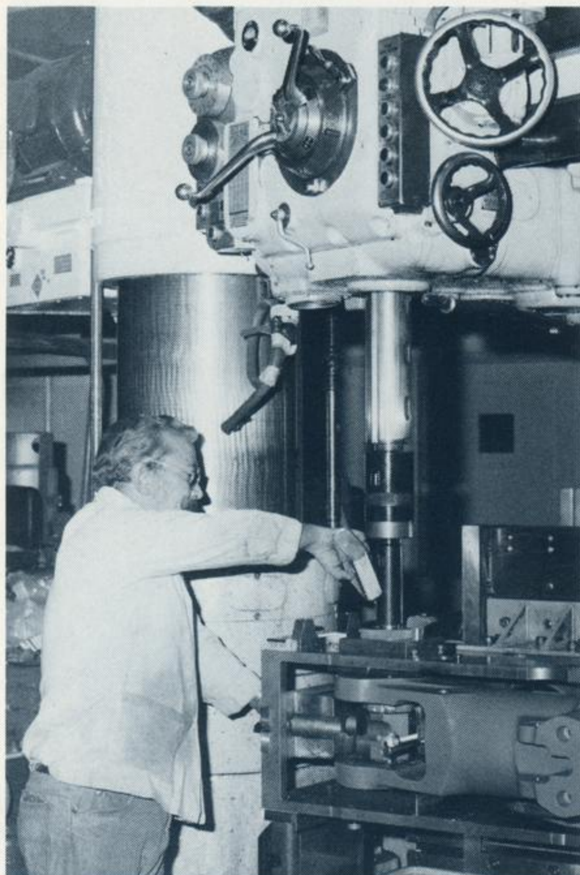
Harold Scholar performs the final reaming process for the grip on a radial drill press.
