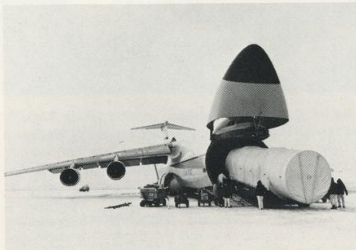
one stage of launch vehicle is loaded aboard a U.S. Air Force C5A cargo jet. Inside C5A
