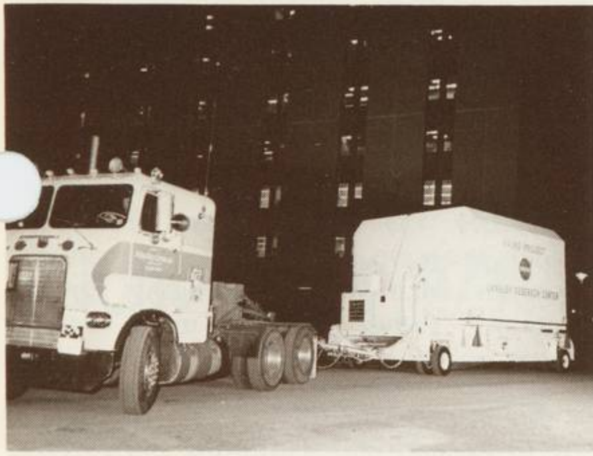
THE VIKING II SPACECRAFT, sealed in its specially built shipping container on a trailer truck, moves out of the space center, on its way to the NASA Kennedy Space Center in Florida. Controls automatically regulate the temperature and humidity around the spacecraft and provide a smooth ride on the 2,100 mile four-day journey.
