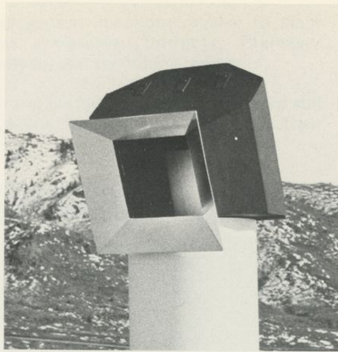
Demonstrating one of the uses of solar energy, this scale model of a boiler/superheater uses the sun's rays to heat water, making steam to drive an electrical generator. Martin Marietta is proposing to build the device and conduct a test program in France.
