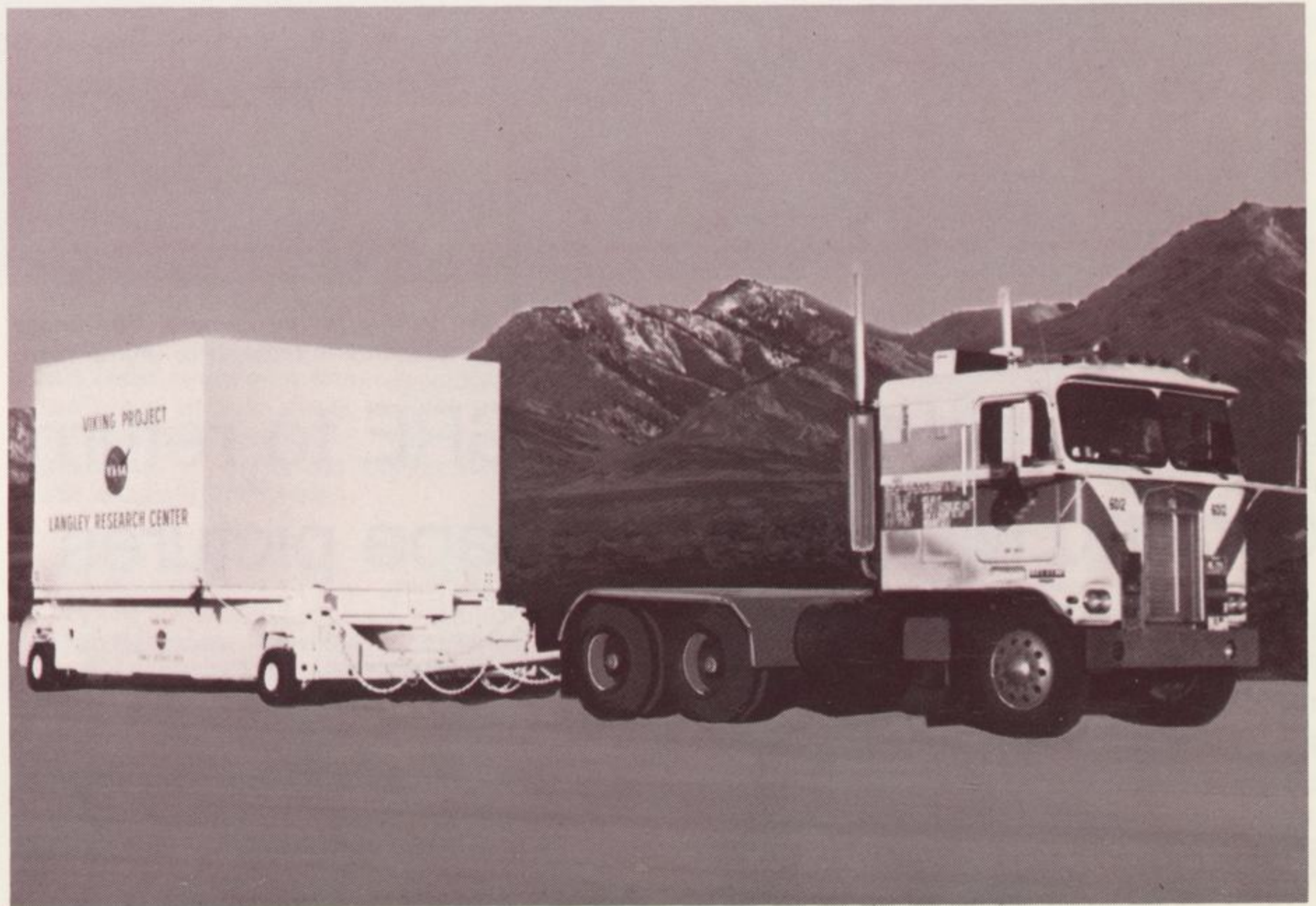
When fully loaded for their trips to Kennedy Space Center in Florida, transporters carrying the Viking lander capsules will weigh 16,000 pounds and carry a self-powered environmental
